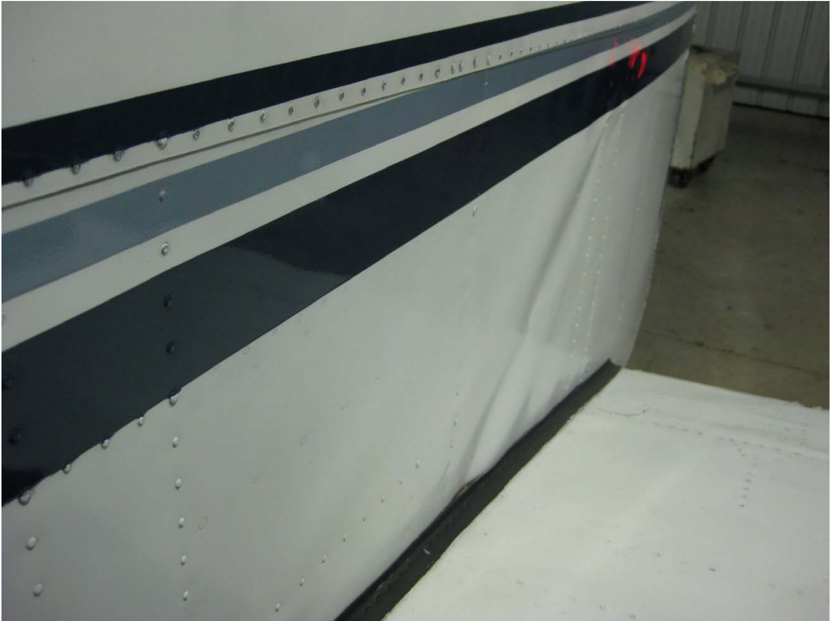
Photo 3 – Deformation in fuselage above wing root.
