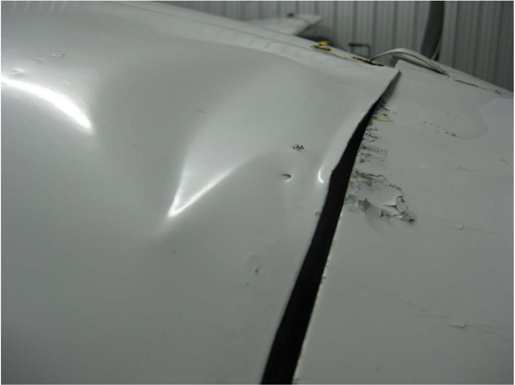
Photo 2 – Damage to the top of the cowling.
