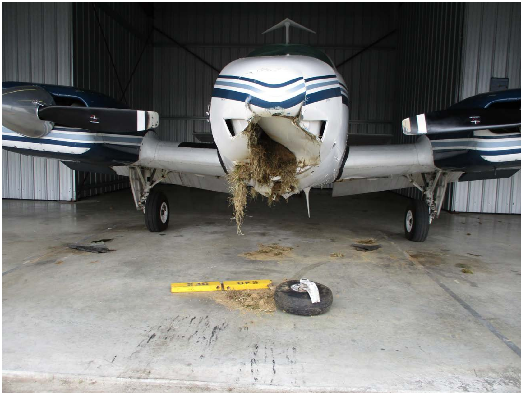
Photo 1 – Front view of airplane with portion of separated nose landing gear.
