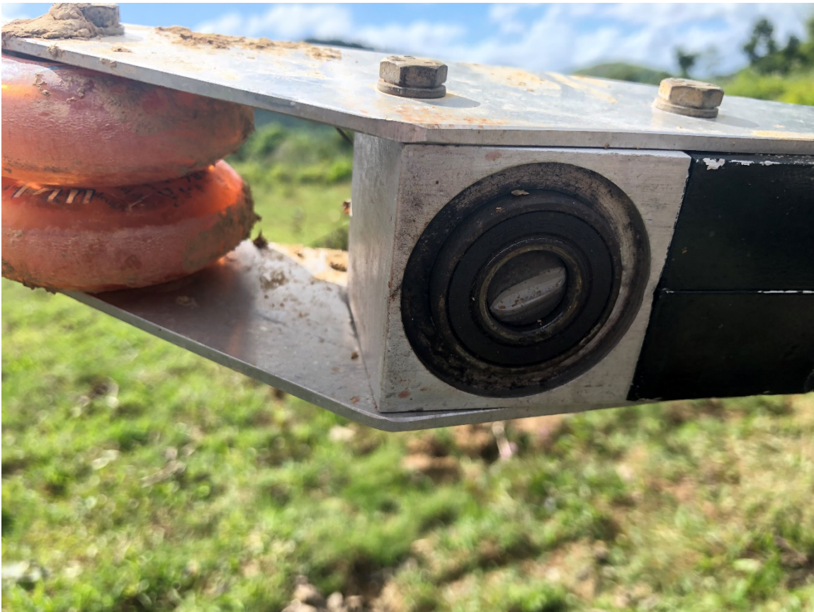
Figure 1. View of Fractured Bolt at Accident Site
