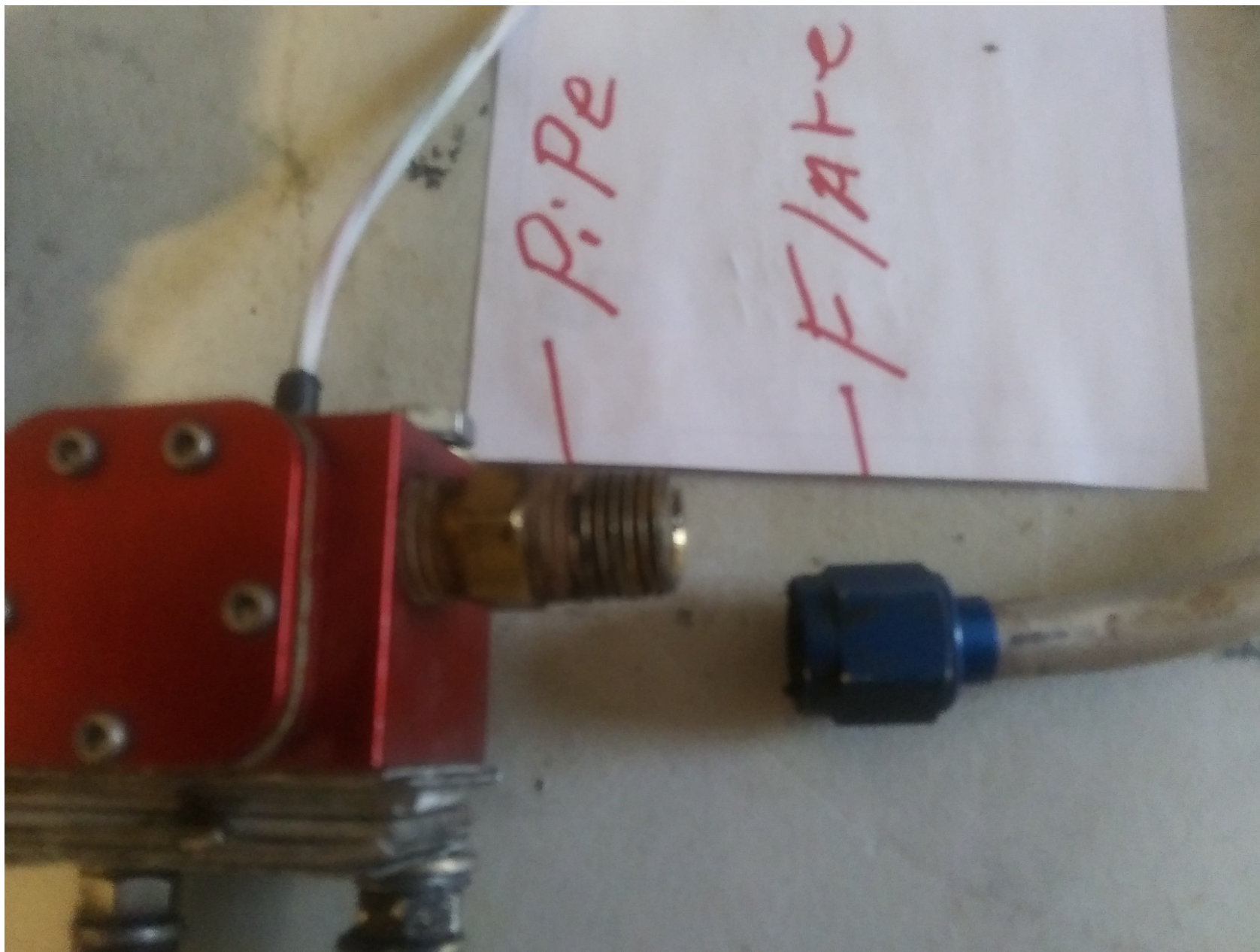
Photo 5 – close-up of pipe fitting connected to flare fitting.
