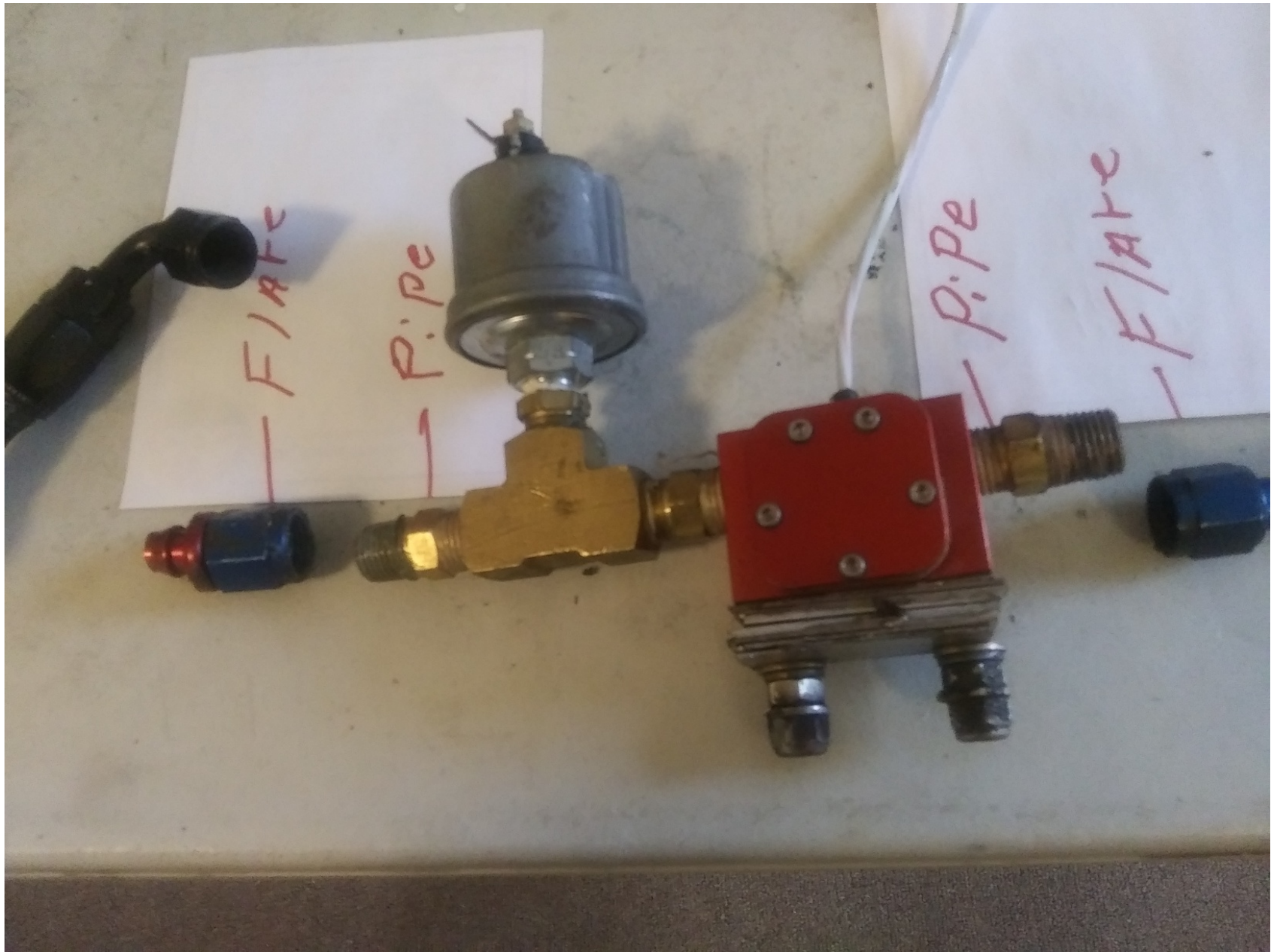
Photo 4 – pipe fittings connected to flare fittings
