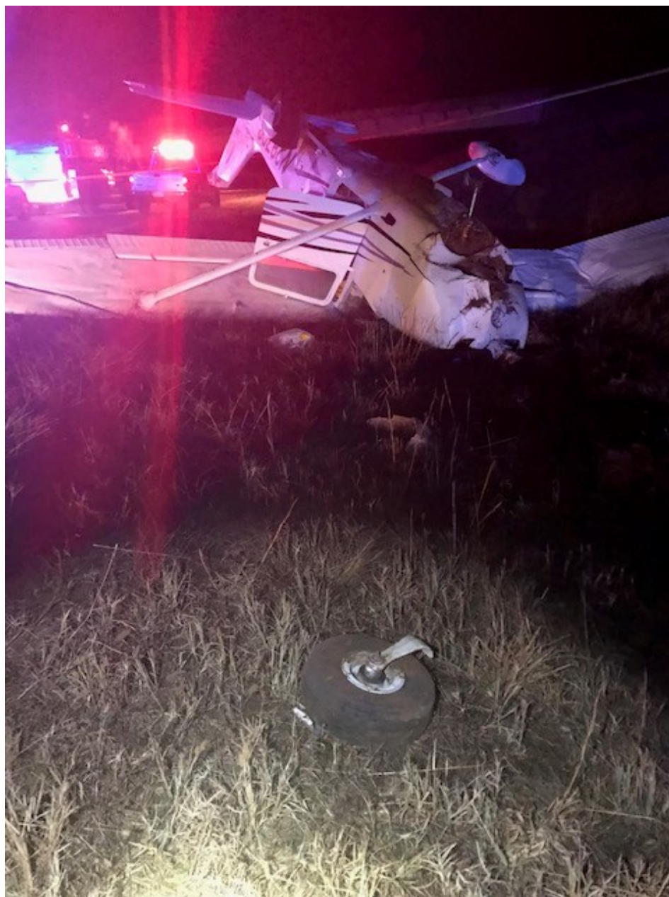
Photo 2 – Front quarter view looking aft. Note damage to fuselage and right wing. (Courtesy of FAA)
