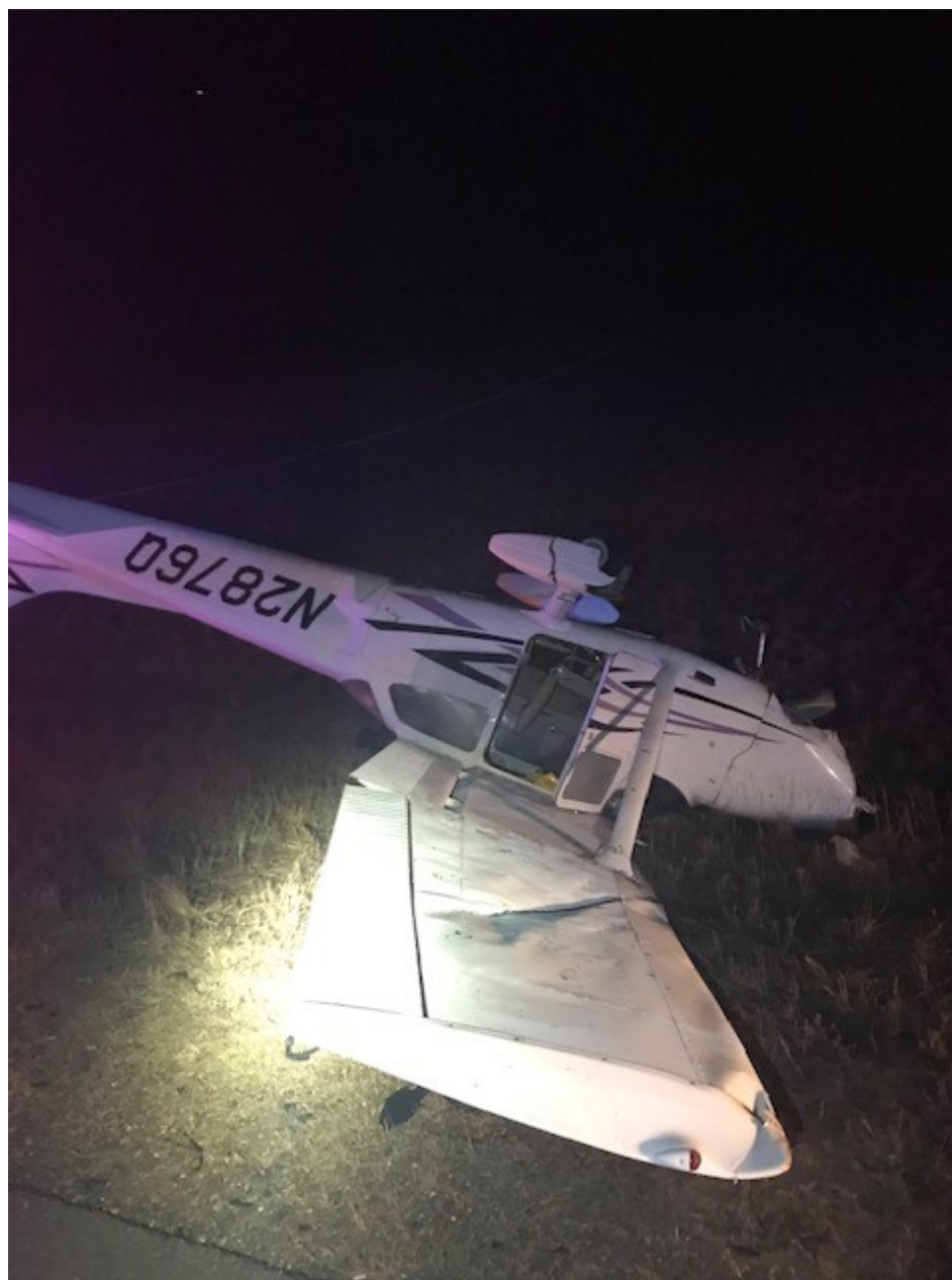
Photo 1 – Left side profile view of inverted airplane damage to left wing. (Courtesy of FAA)
