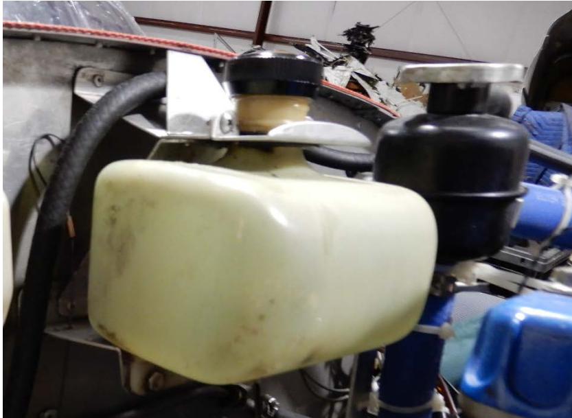
Figure 5. View of oil injection tank as found. Note: no oil.
