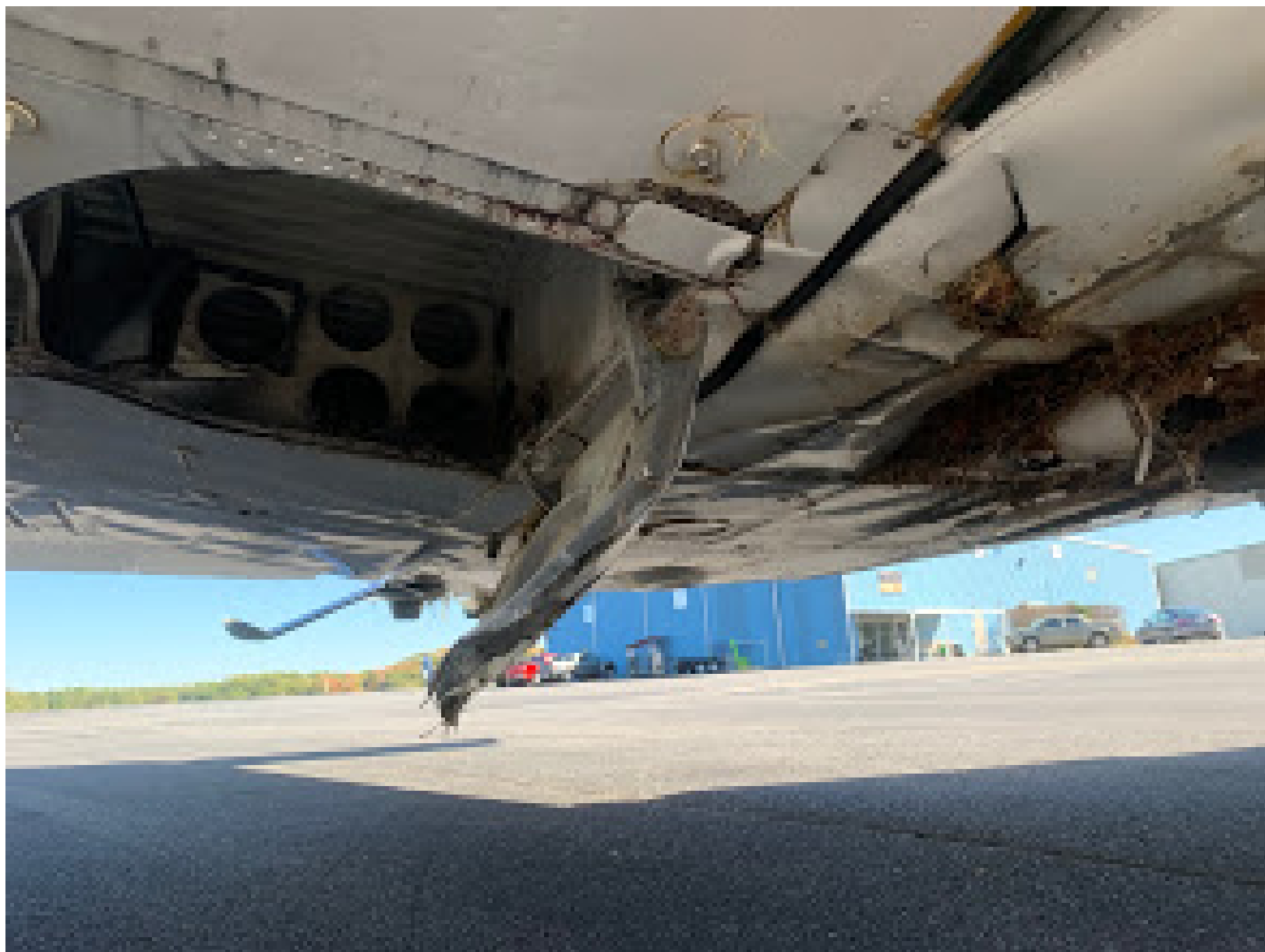
Photo 3 – View of damage to fuselage and right landing gear door. (Courtesy of FAA)
