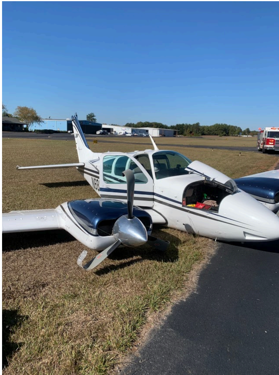
Photo 1 – View of right front quarter of airplane at rest on the side of the runway. Note gear up configuration and propeller damage. (Courtesy of FAA)
