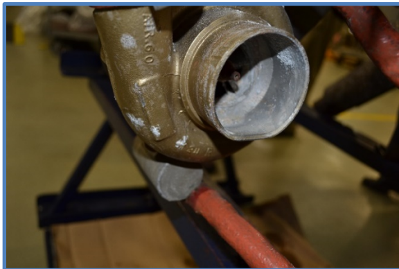
Picture 6. View damaged right turbo
