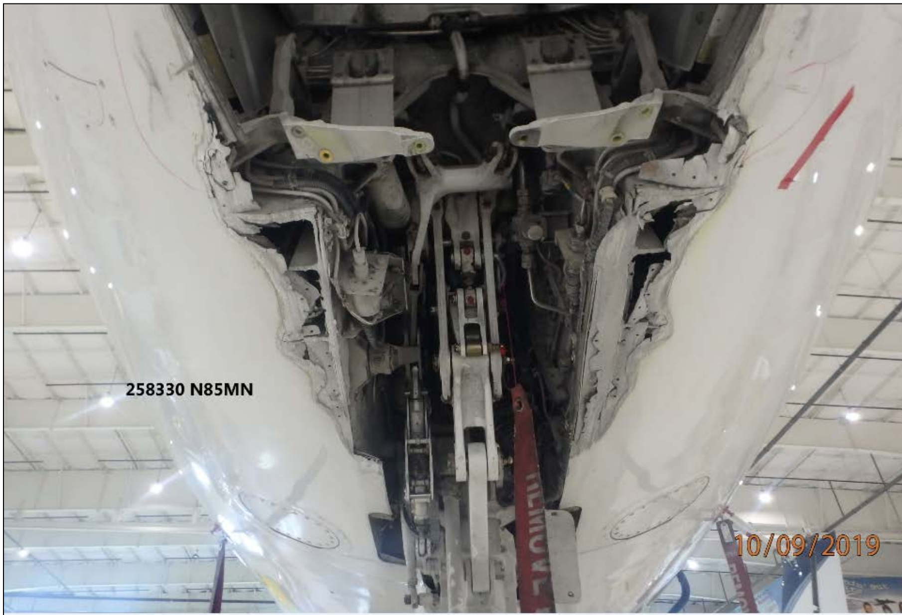
Photo 3 – View of the substantially damaged fuselage (Photograph Courtesy of Delta Private Jets)
