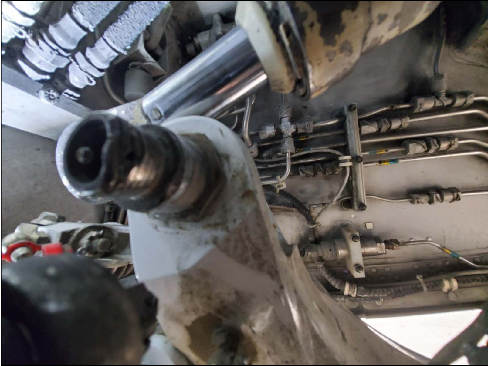
Photo 2 – View of the nose landing gear actuator attachment area (Photograph Courtesy of FAA)
