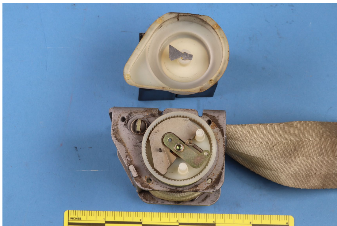
Figure 4: Pilot's seat belt reel with inertial locking mechanism cover removed.
