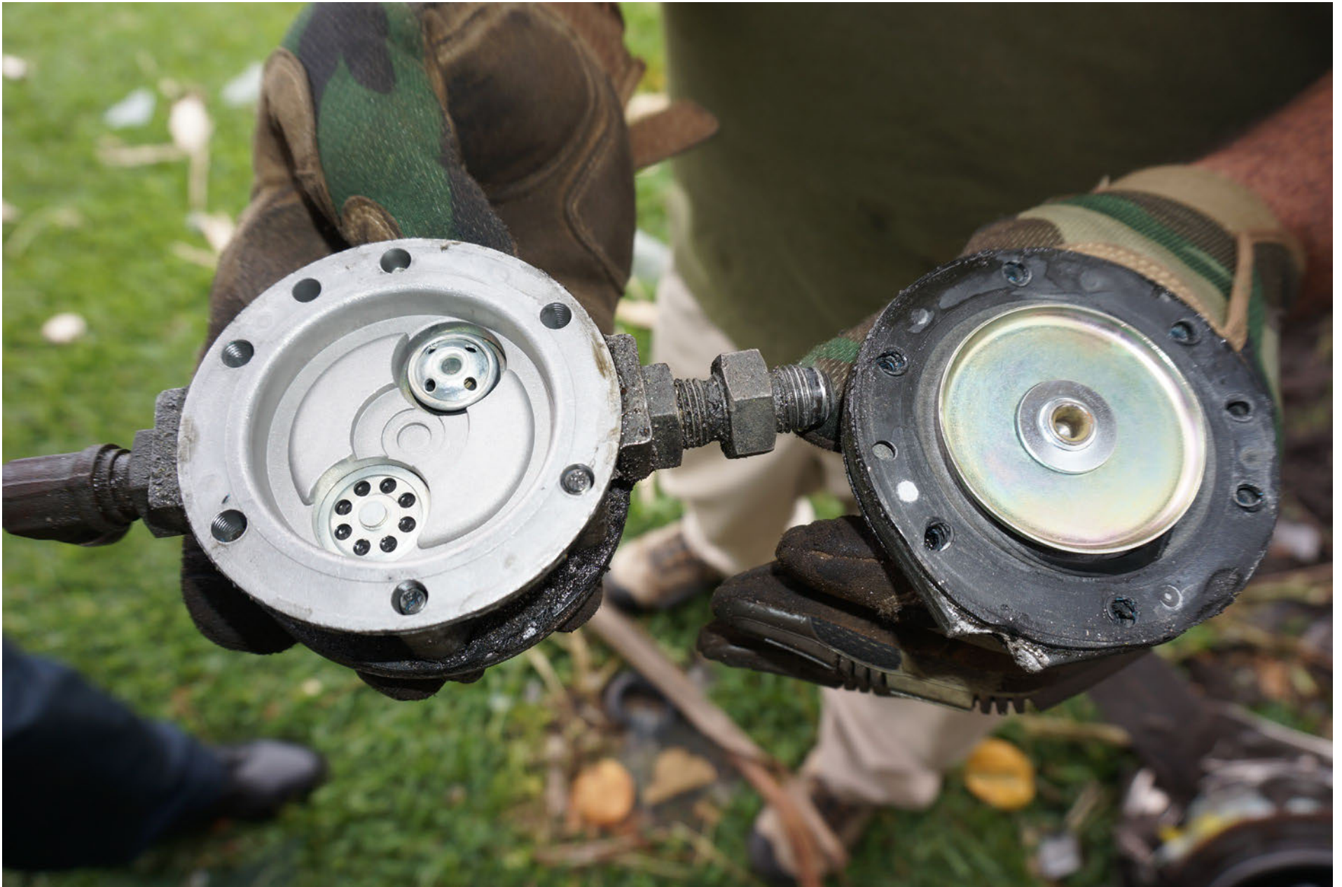
Photo 9 – Engine Driven Fuel Pump
