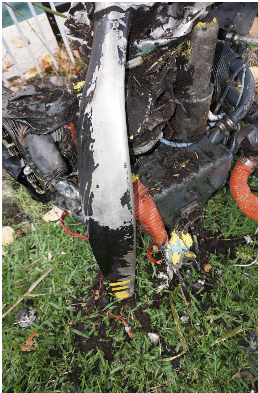
Photo 13 – Bent Back Propeller Blade
