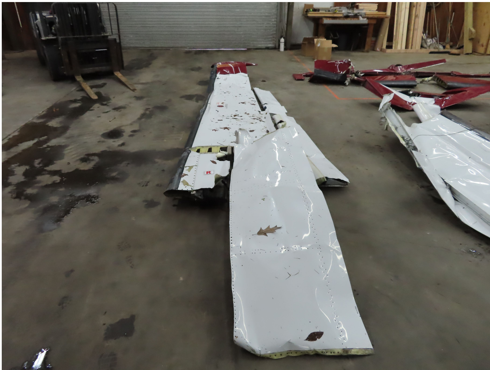
Photo 4 – View of portions of the right wing. (Photo courtesy of Piper)
