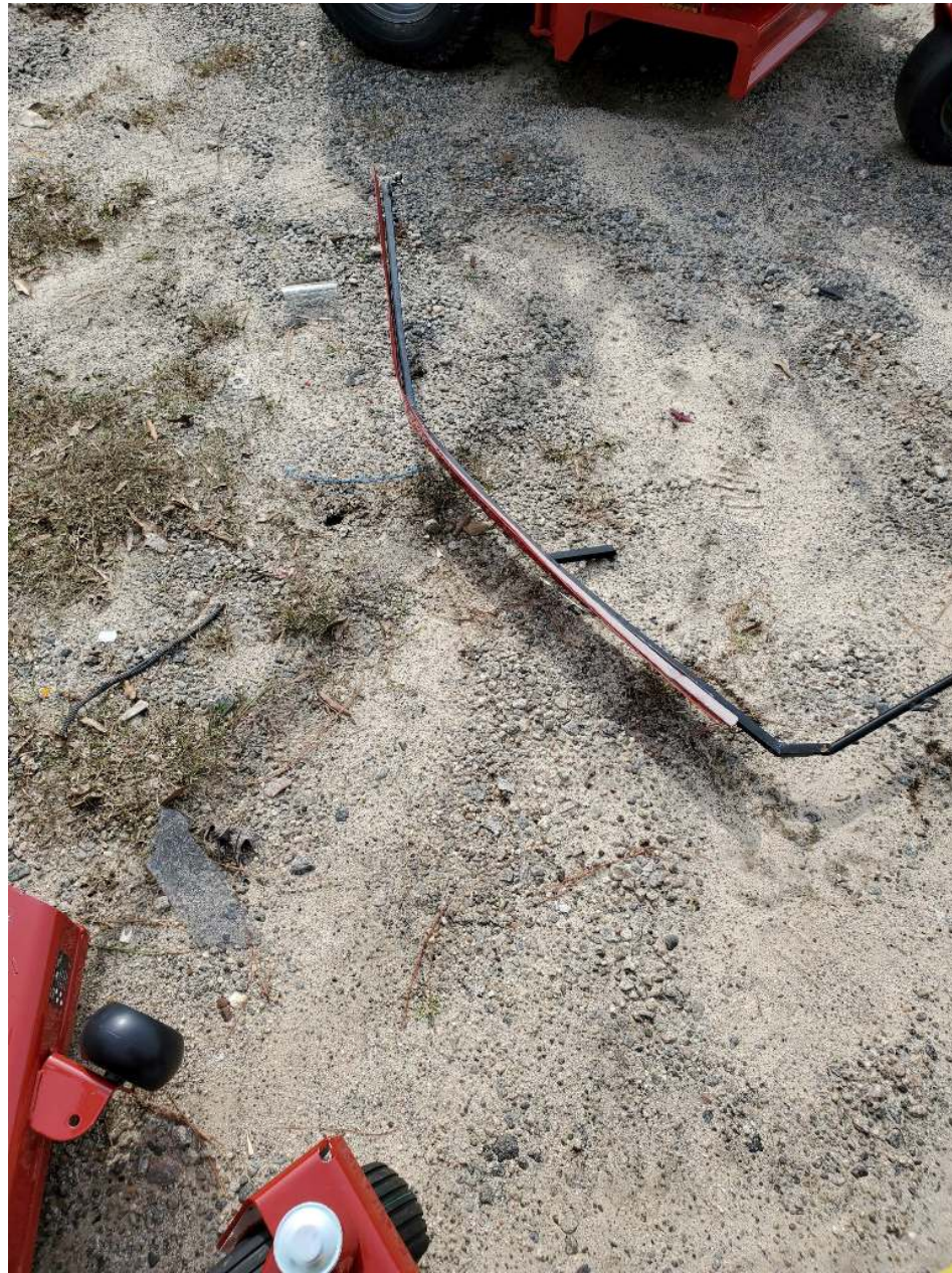
Photo 3 – Section of Canopy Frame (Photo Courtesy of FAA)
