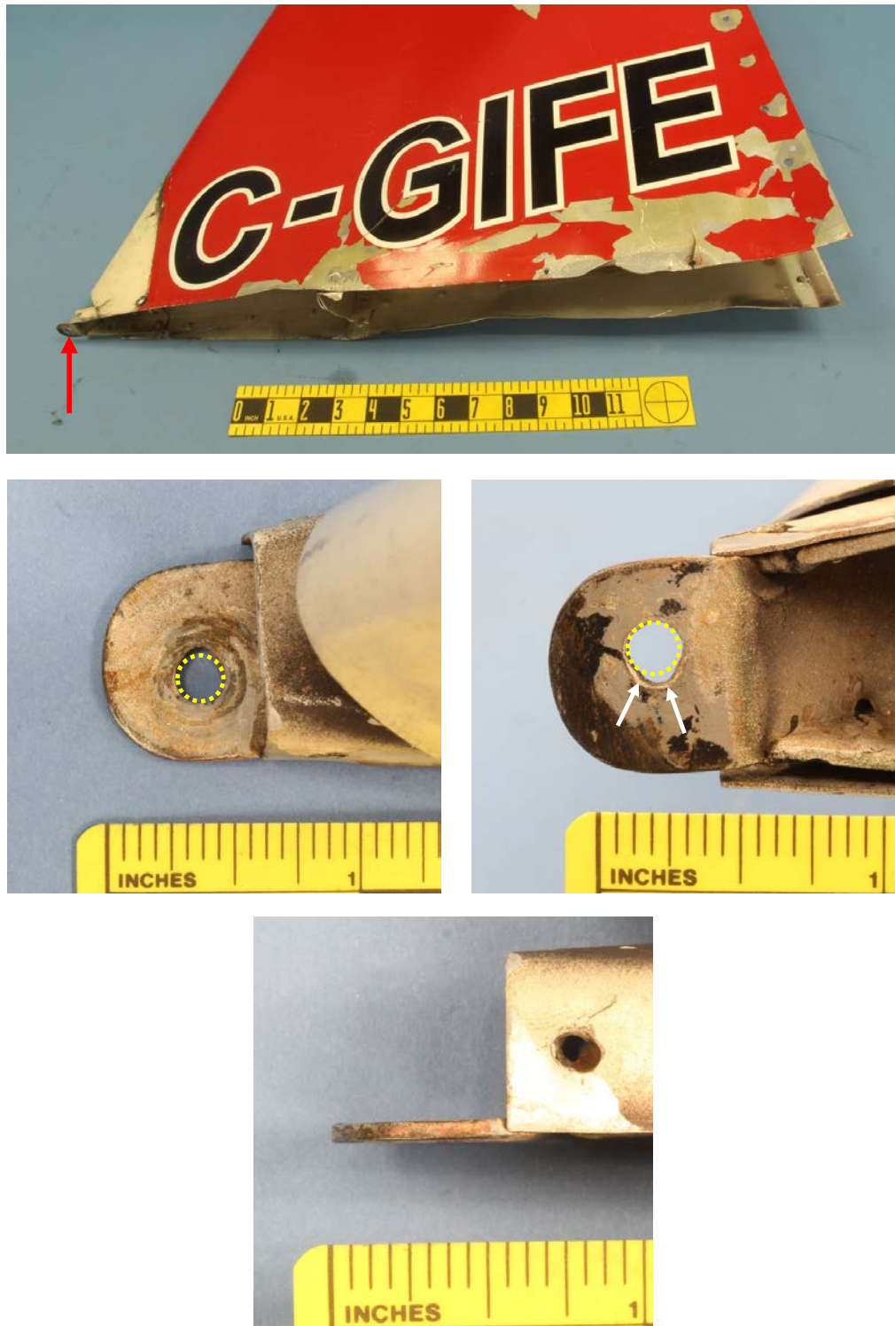
Figure 9: Close-up photos of the forward attach point (red arrow, top photo) on the vertical stabilizer. The top and bottom of the attach point bolt hole are shown in the center left and right photos, respectively. The yellow dotted lines illustrate a round bolt hole. The white arrows point to rolled material. The bottom photo shows a profile view of the attach point.
