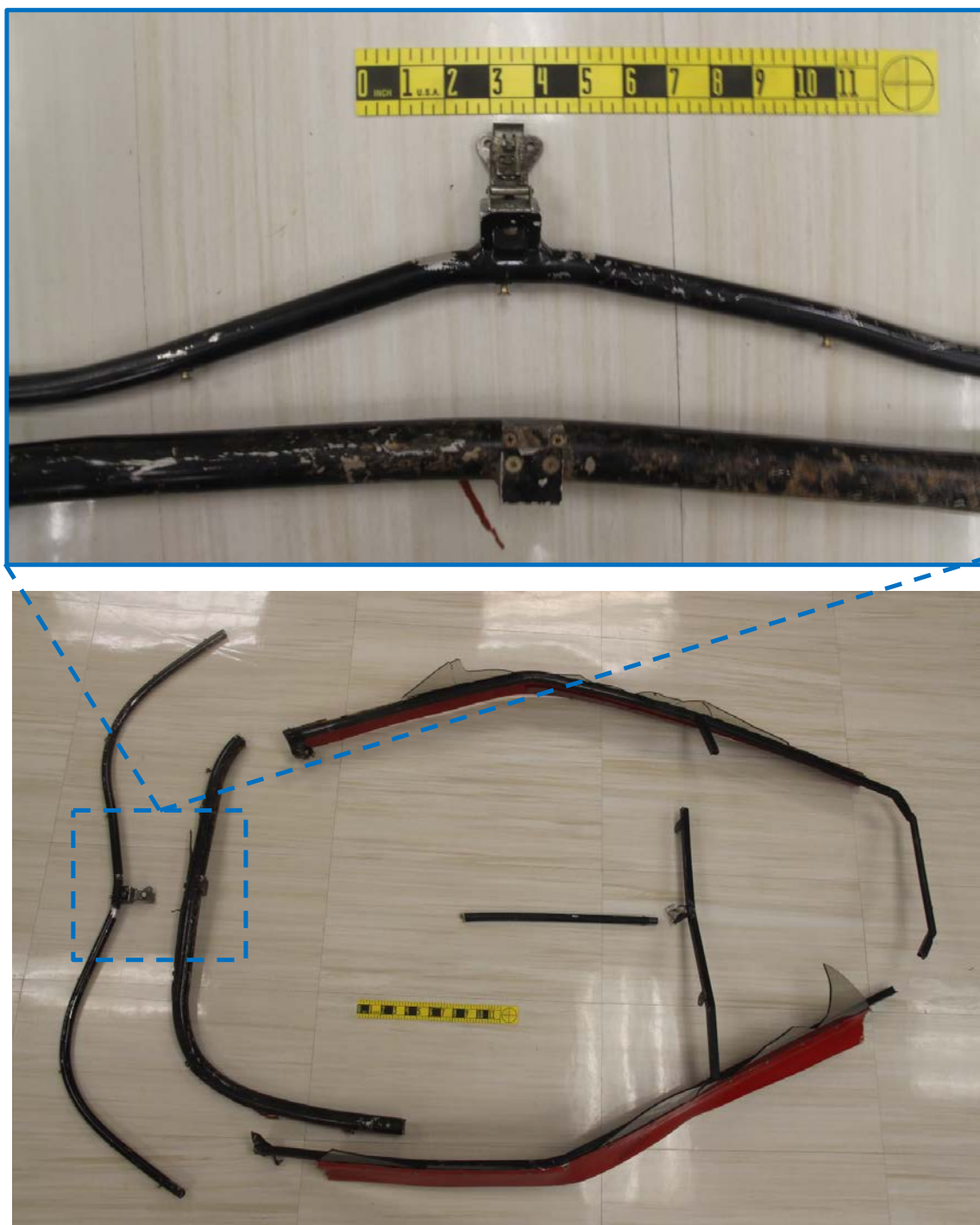
Figure 4: The bottom shows an overall photo of the canopy frame pieces, and the top shows a close-up photo of the canopy locking mechanism.
