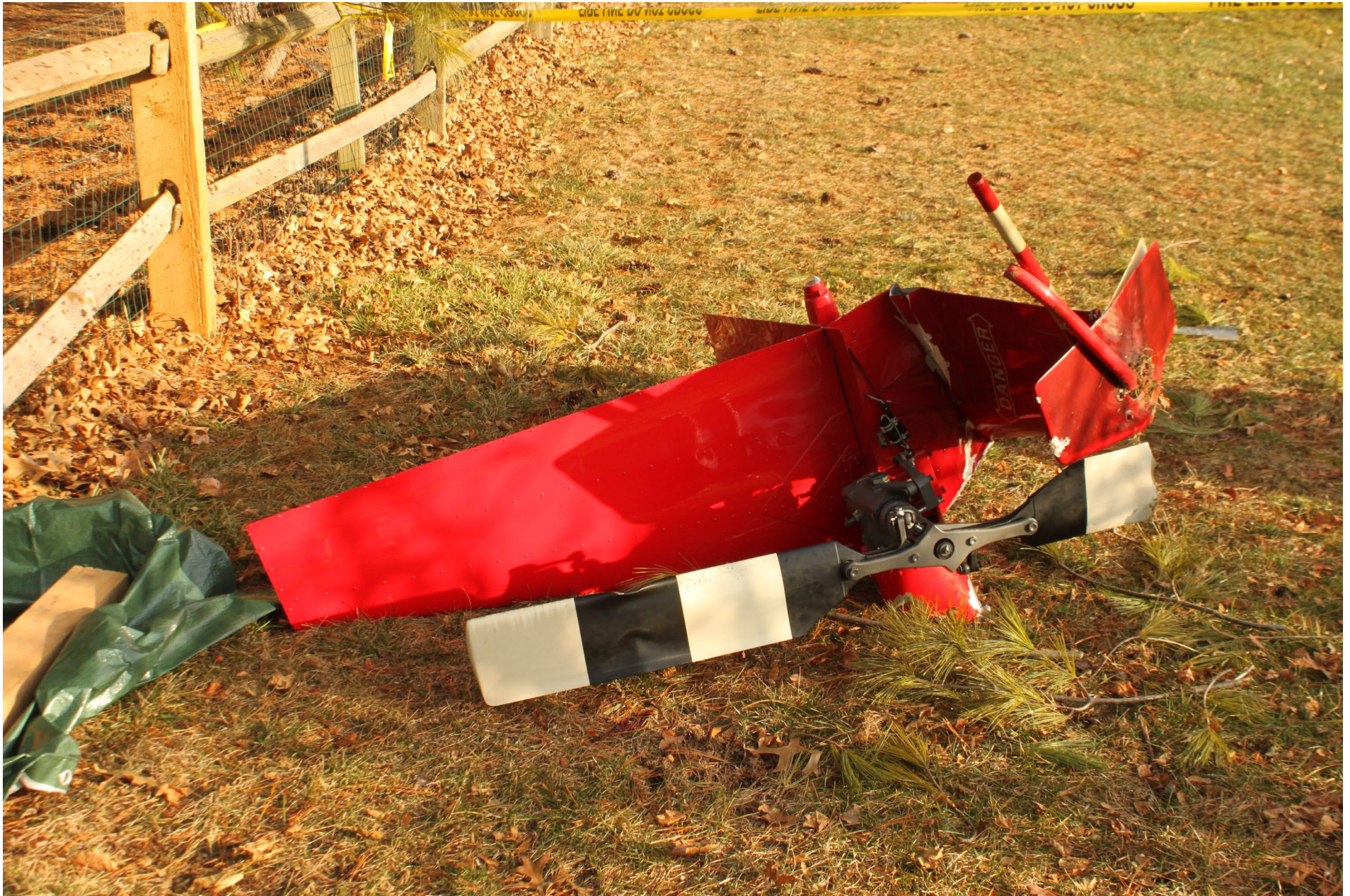
Photo 5 - NTSB Digital Photograph. View of the Separated Tail Rotor Assembly. Note the fractured Tail Rotor Blade.
