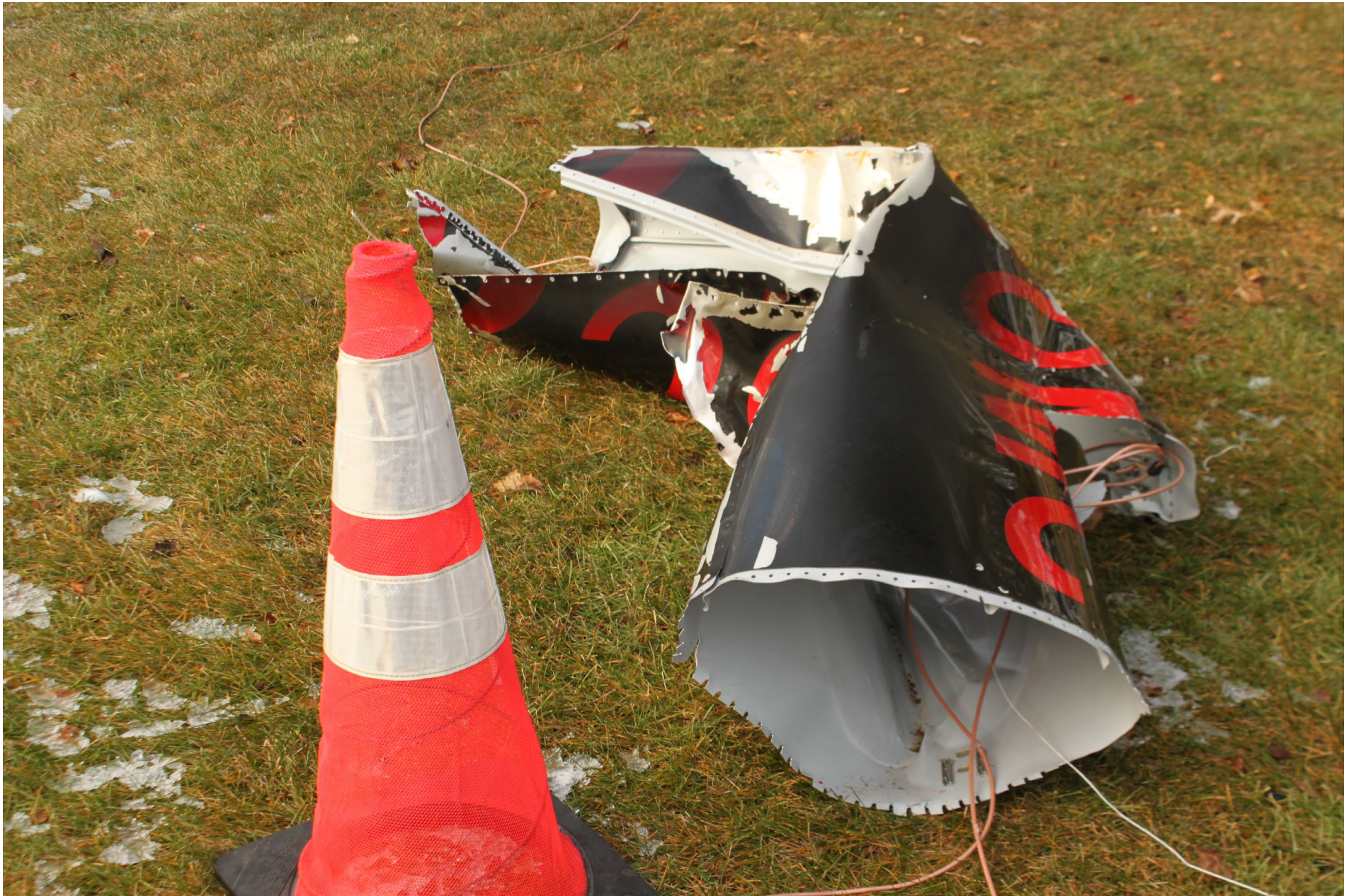
Photo 7 - NTSB Digital Photograph. View of a Portion of the Separated Tailboom.
