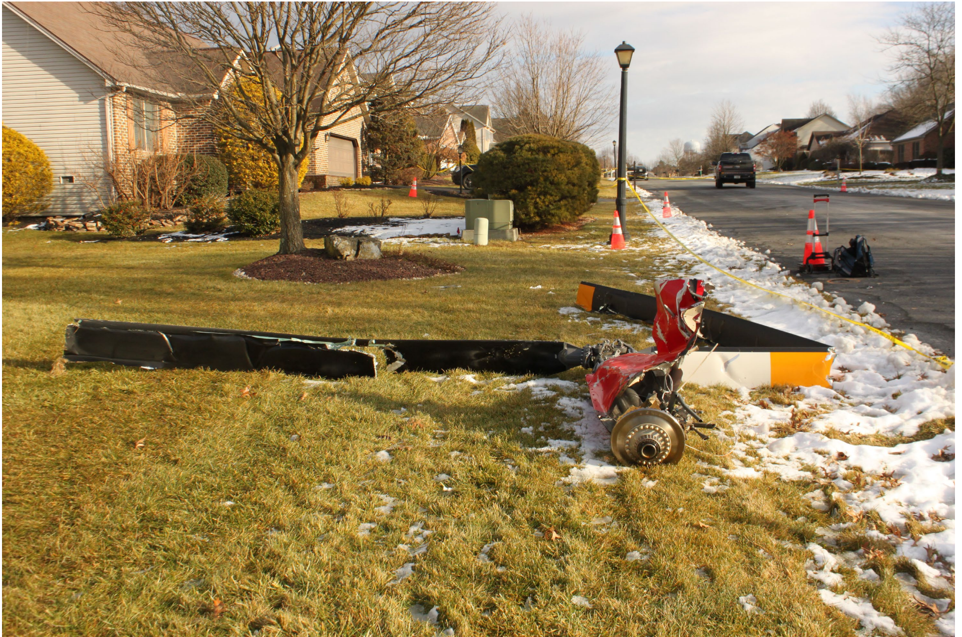
Photo 3 - NTSB Digital Photograph. Different View of the Separated Main Rotor Mast with Attached Main Rotor Blades.
