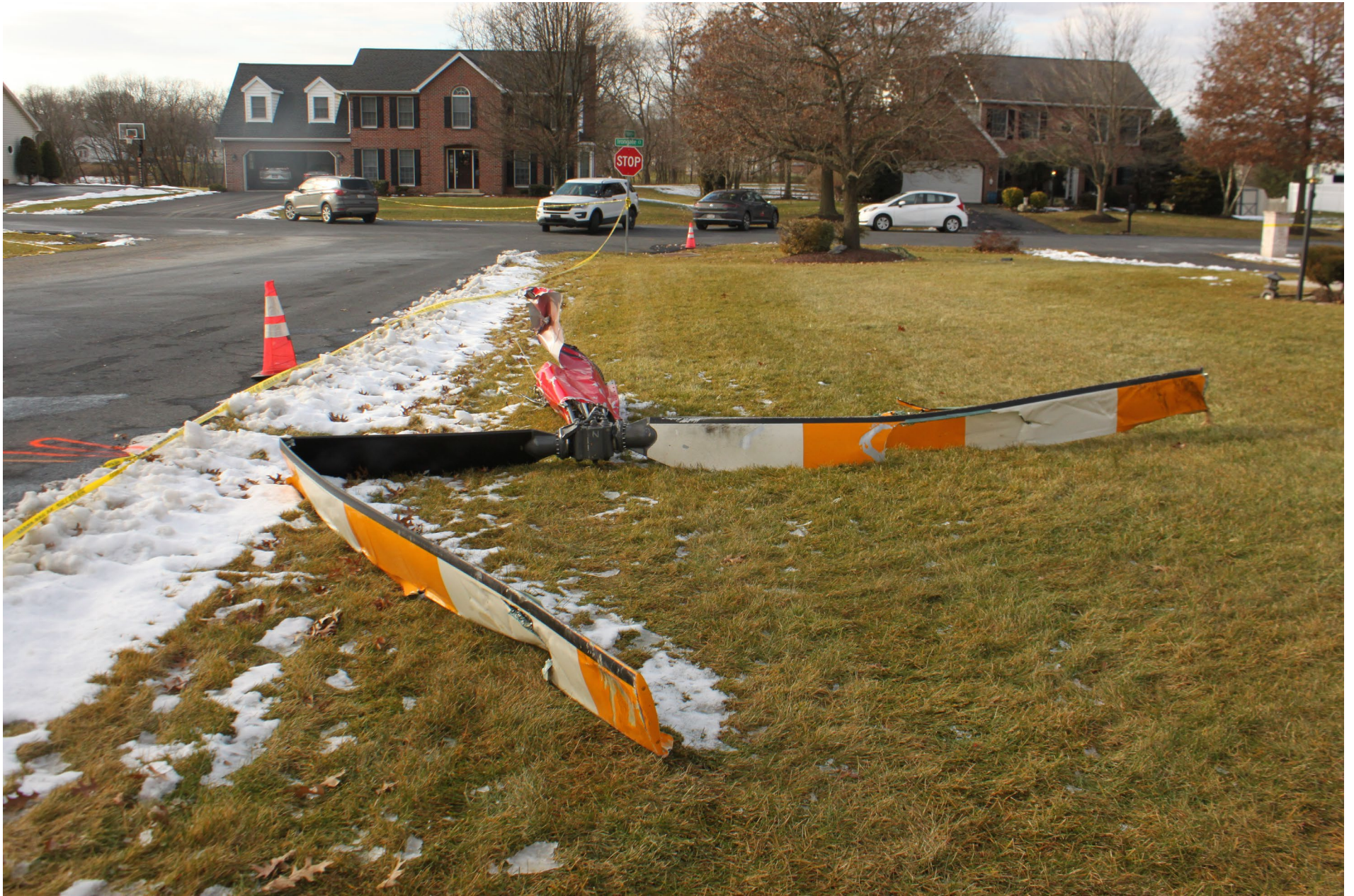
Photo 2 - NTSB Digital Photograph. View of the Separated Main Rotor Mast with Attached Main Rotor Blades.
