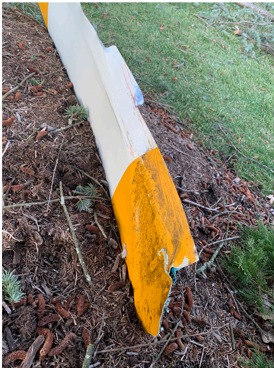
Photo 9 – FAA Digital Photograph. View of the Inboard Section of the Separated Main Rotor Blade. Note the Feather Adhering to the Upper Surface of the Blade near the Leading Edge.
