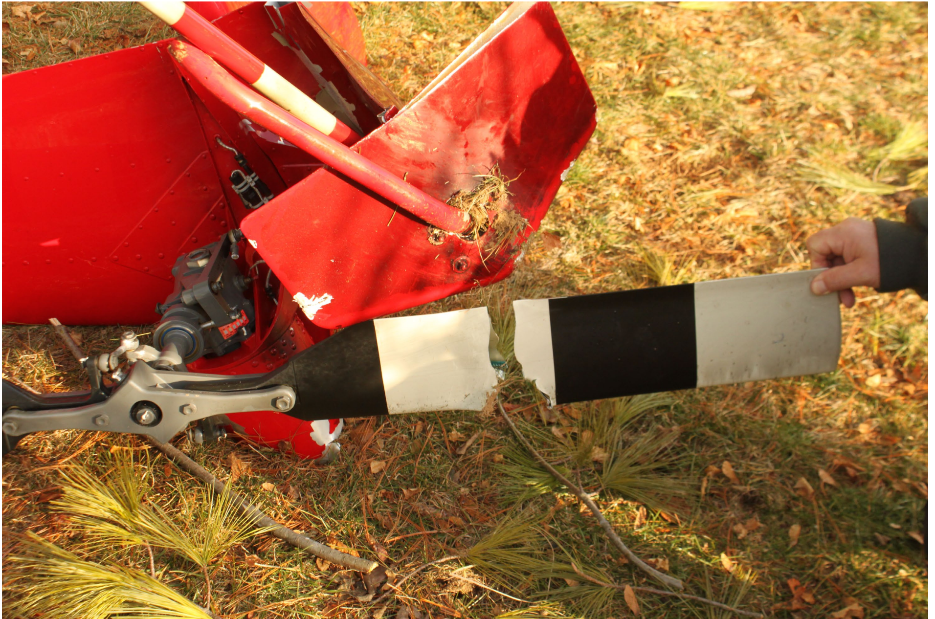
Photo 6 - NTSB Digital Photograph. Close-Up View of the fractured Tail Rotor Blade Showing the recovered Section of Tail Rotor Blade in the Photograph.
