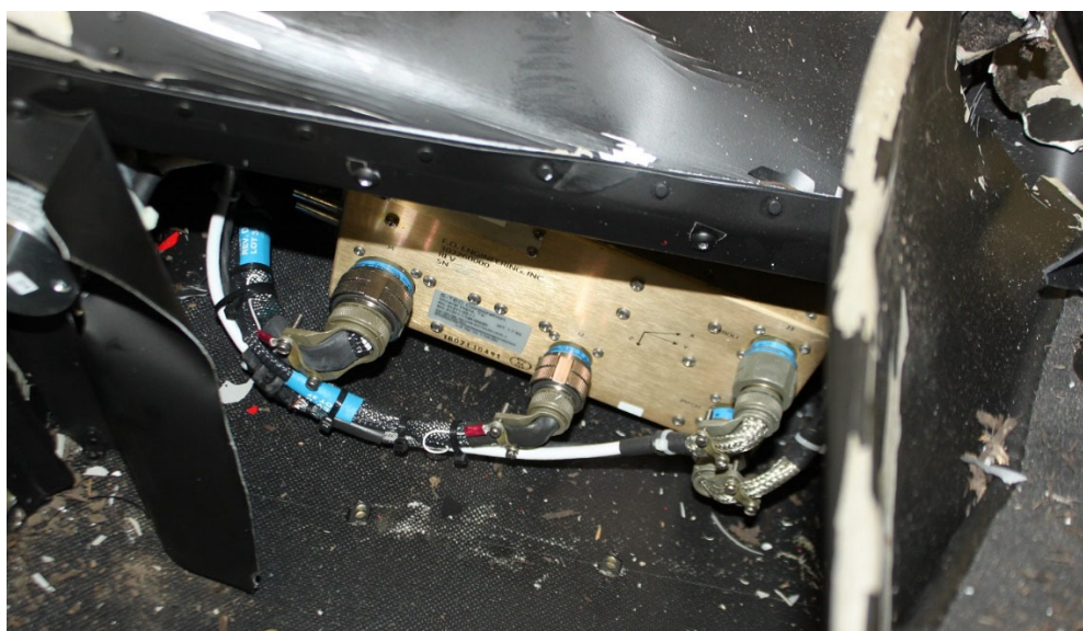
Figure 6. The FCC as seen in the wreckage.
