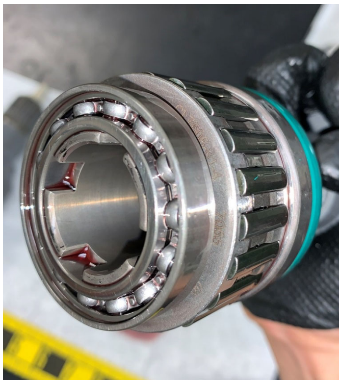
Figure 4. A view of the sprag elements and a bearing.
