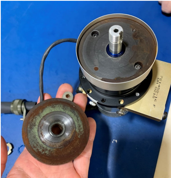
Figure 13. Pitch servo-actuator magnet and friction plate.
