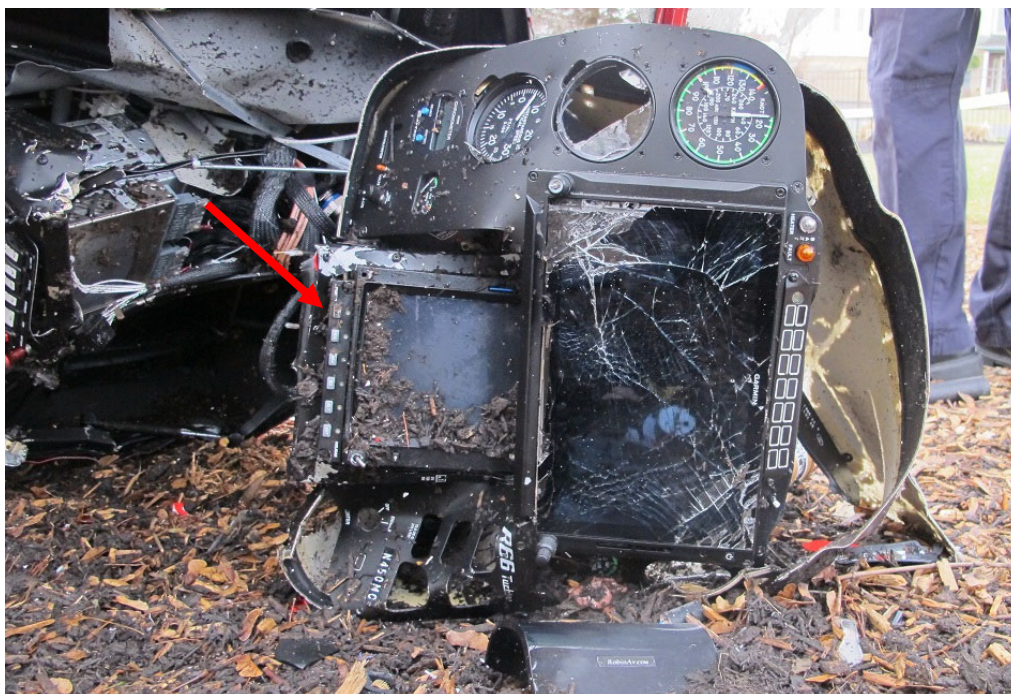
Figure 5. The red arrow points to the HCP installed within the instrument panel. (Image courtesy of Robinson Helicopter Company)
