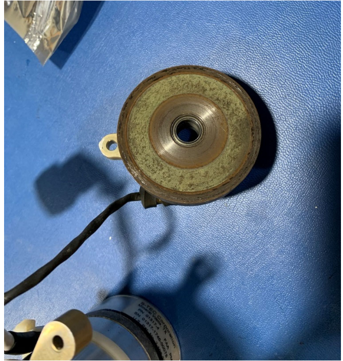
Figure 16. Roll servo-actuator magnet.
