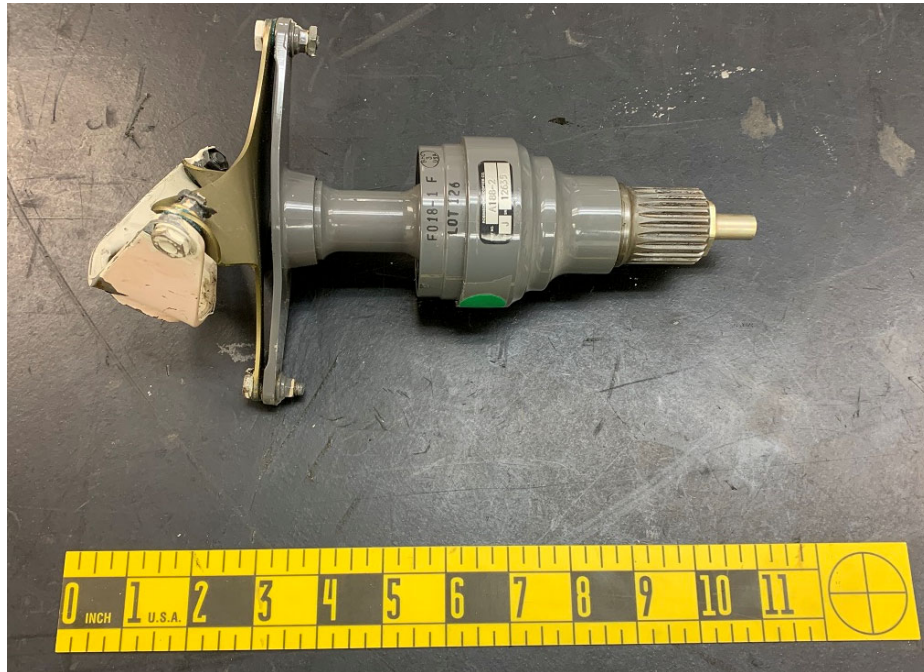
Figure 2. The recovered sprag clutch assembly.
