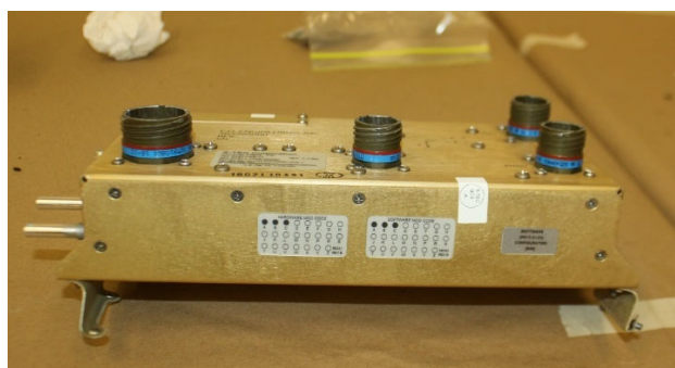
Figure 10. The recovered FCC.
