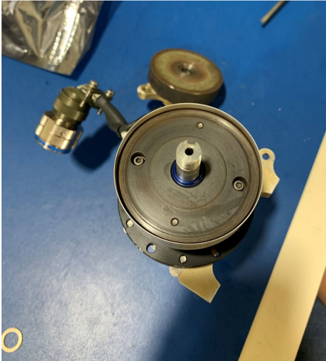
Figure 15. Roll servo-actuator friction plate.
