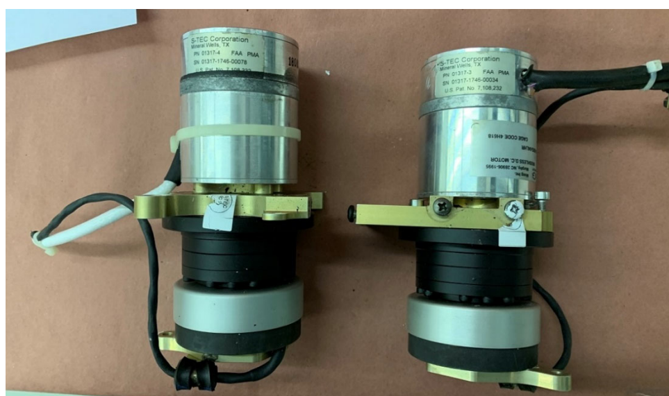
Figure 12. The roll (left) and pitch (right) servo-actuators after removal from the wreckage.
