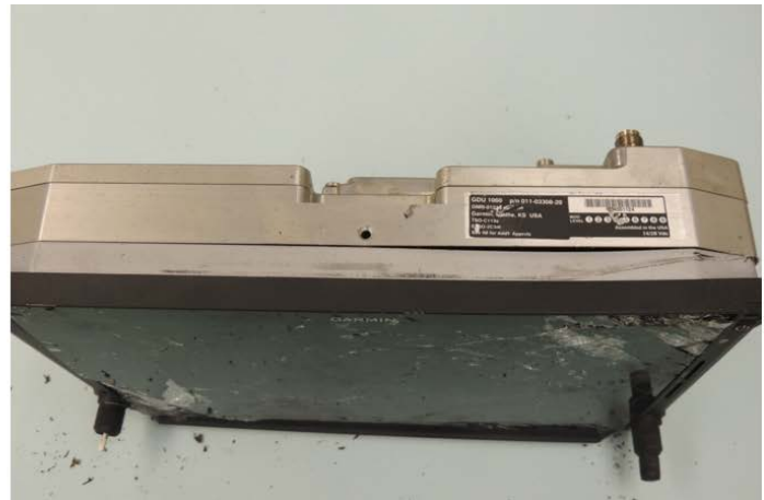
Figure 2: Front and side views of the Garmin GDU 1060 as received.
