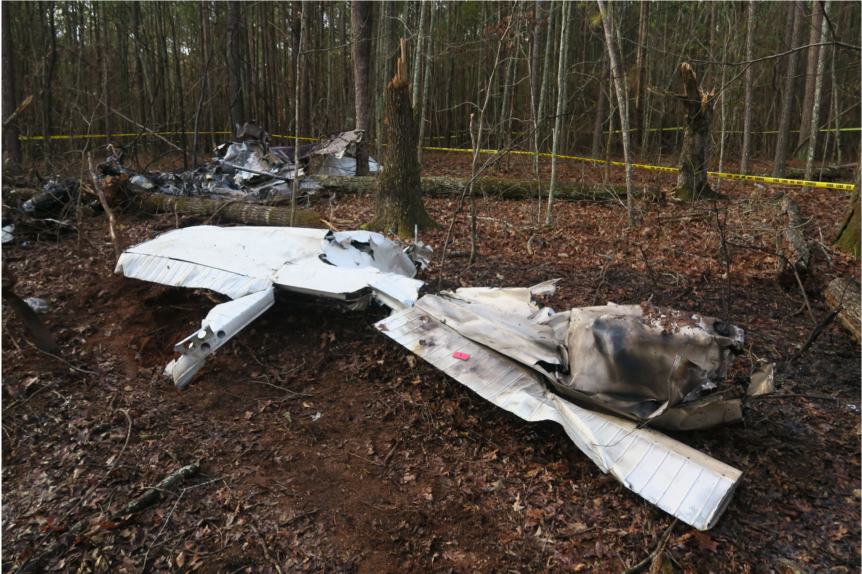
Photo 9 – View of separated left wing as discovered at the accident site; about 20 feet from the main wreckage.
