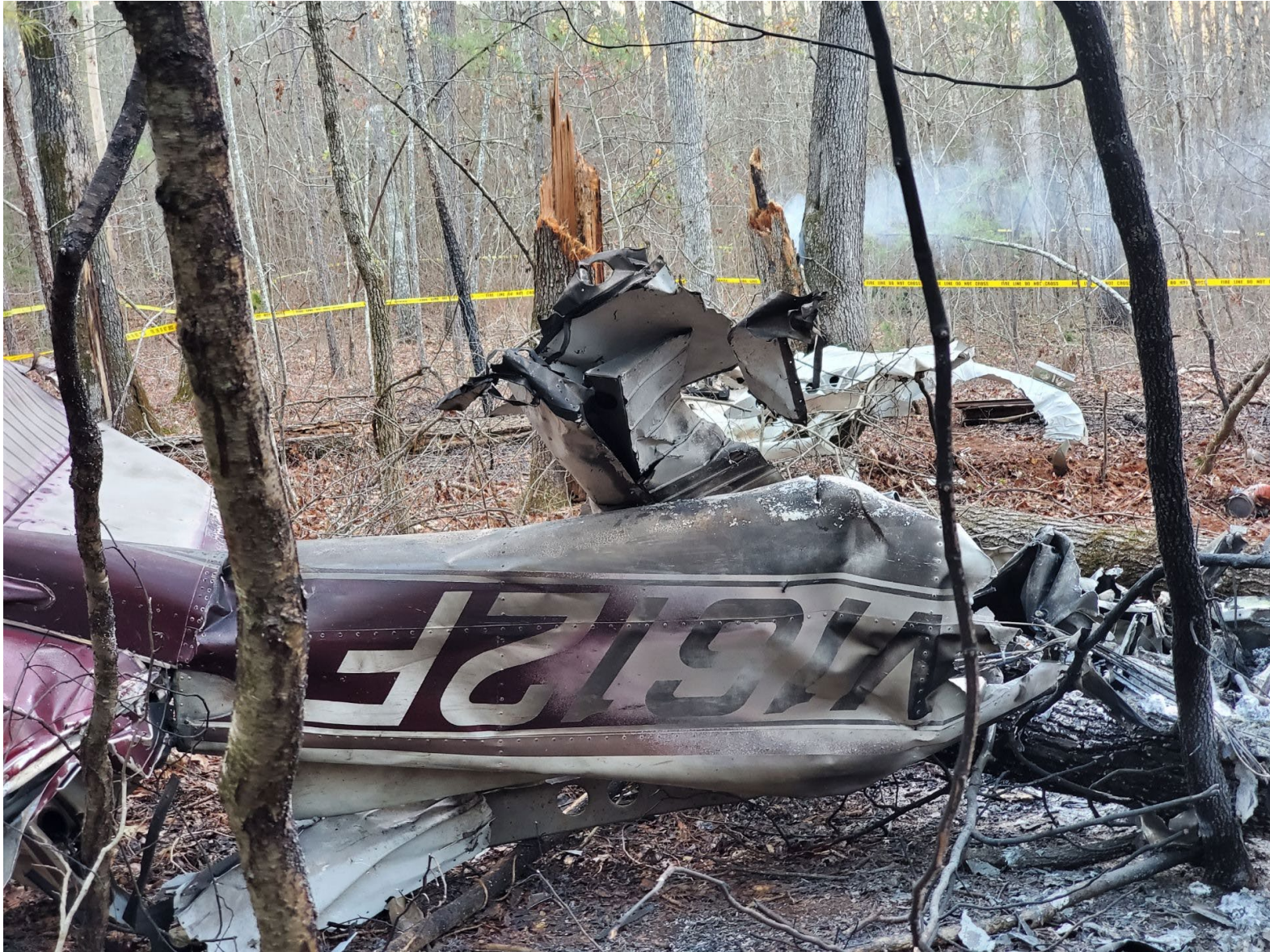
Photo 2 – Close up view of fuselage damage looking towards the initial impact site that originated about 180 ft in the background.
