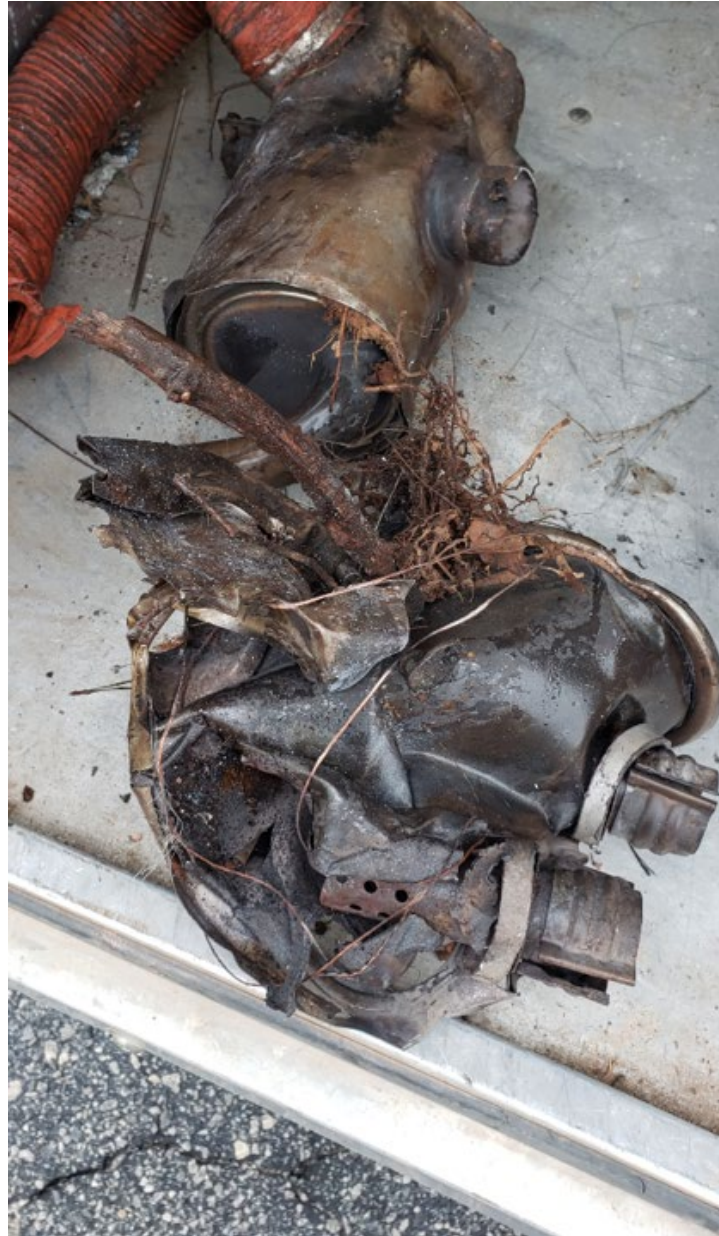
Photo 12 – View of left and right muffler assemblies after recovery from site.
