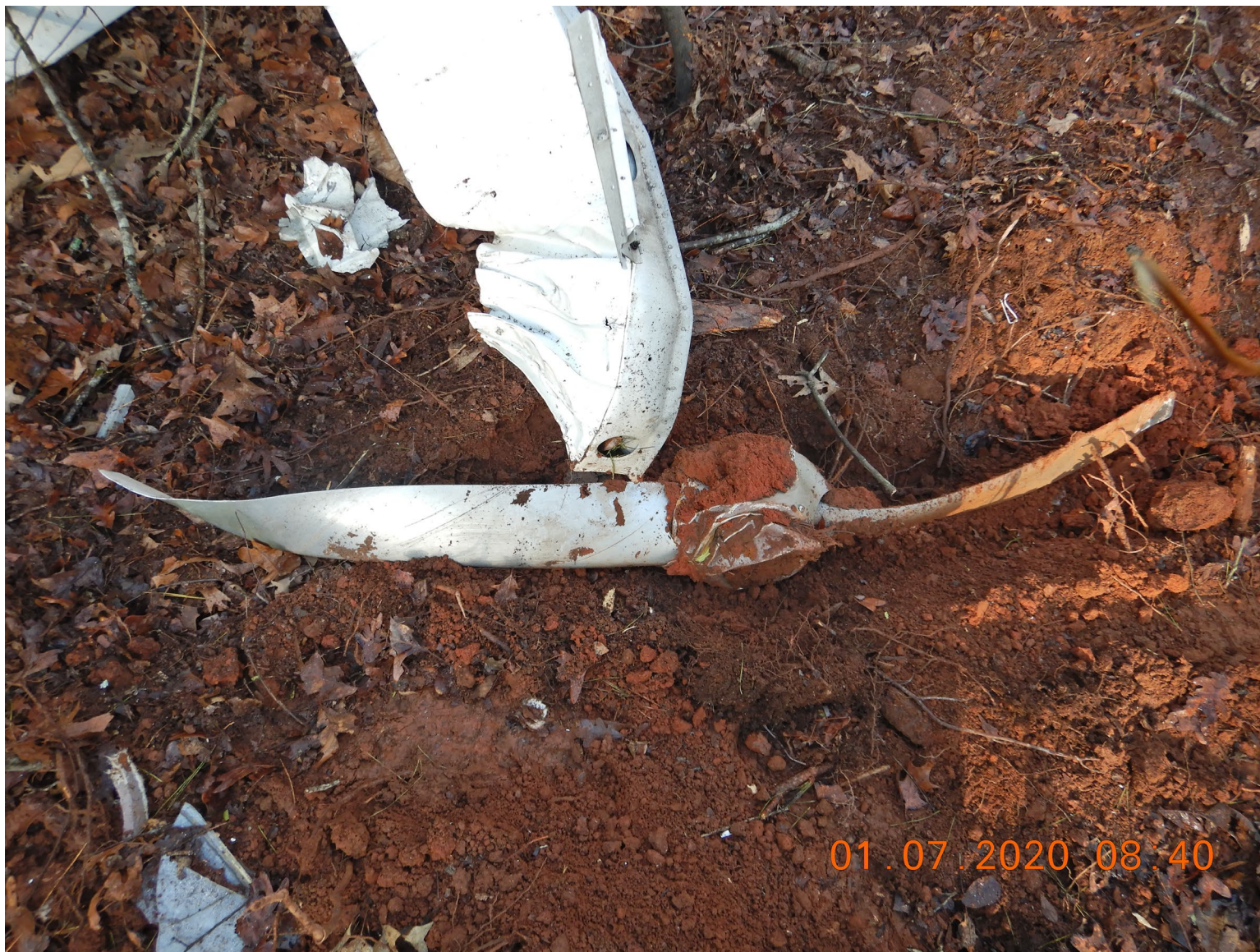
Photo 7 – View of separated propeller after removal from the ground.
