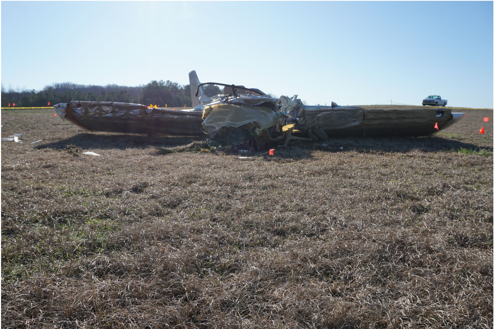
Photo 3 – Forward view of airplane showing crush damage.
