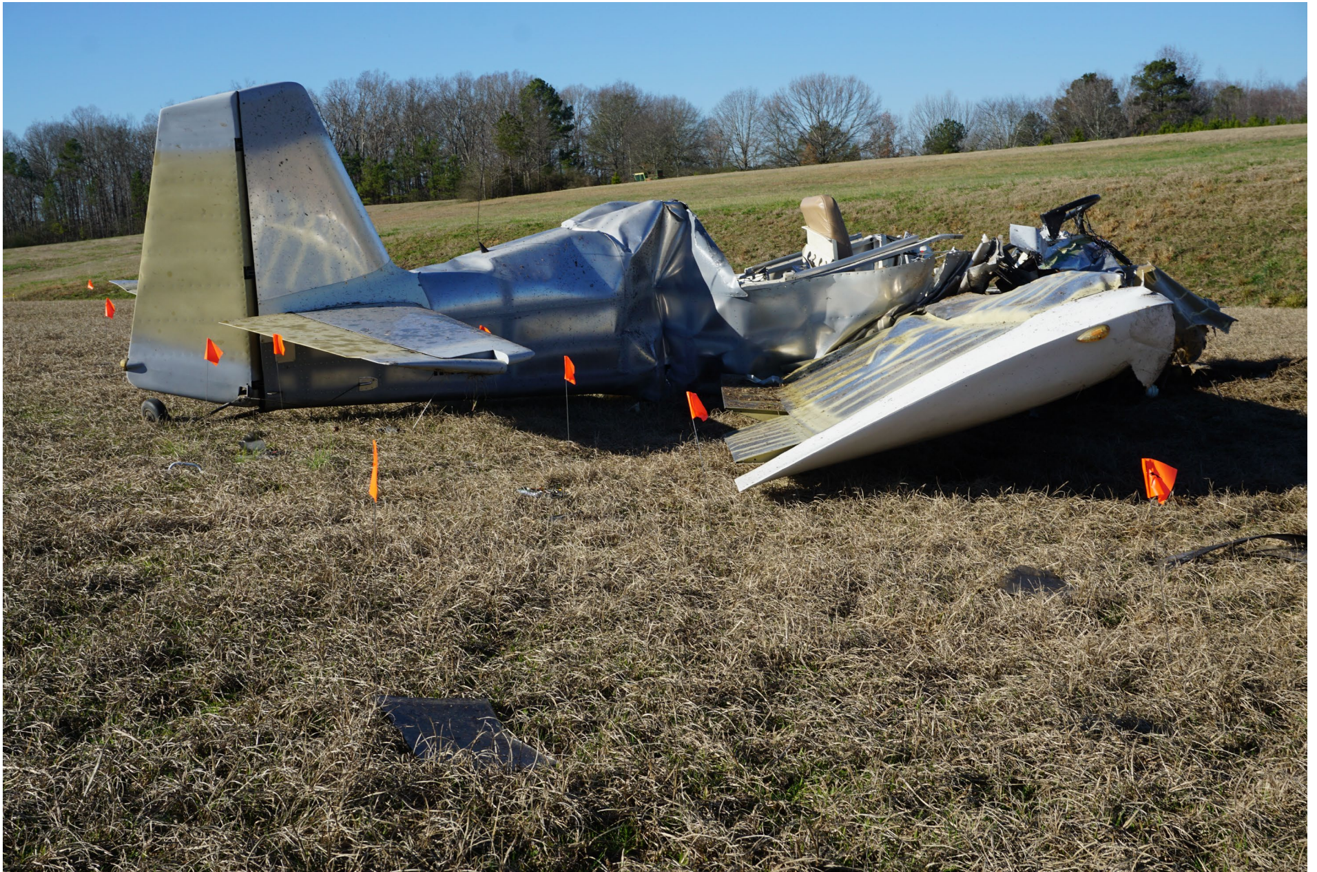
Photo 2 – Right-side view of airplane showing right wing damage.
