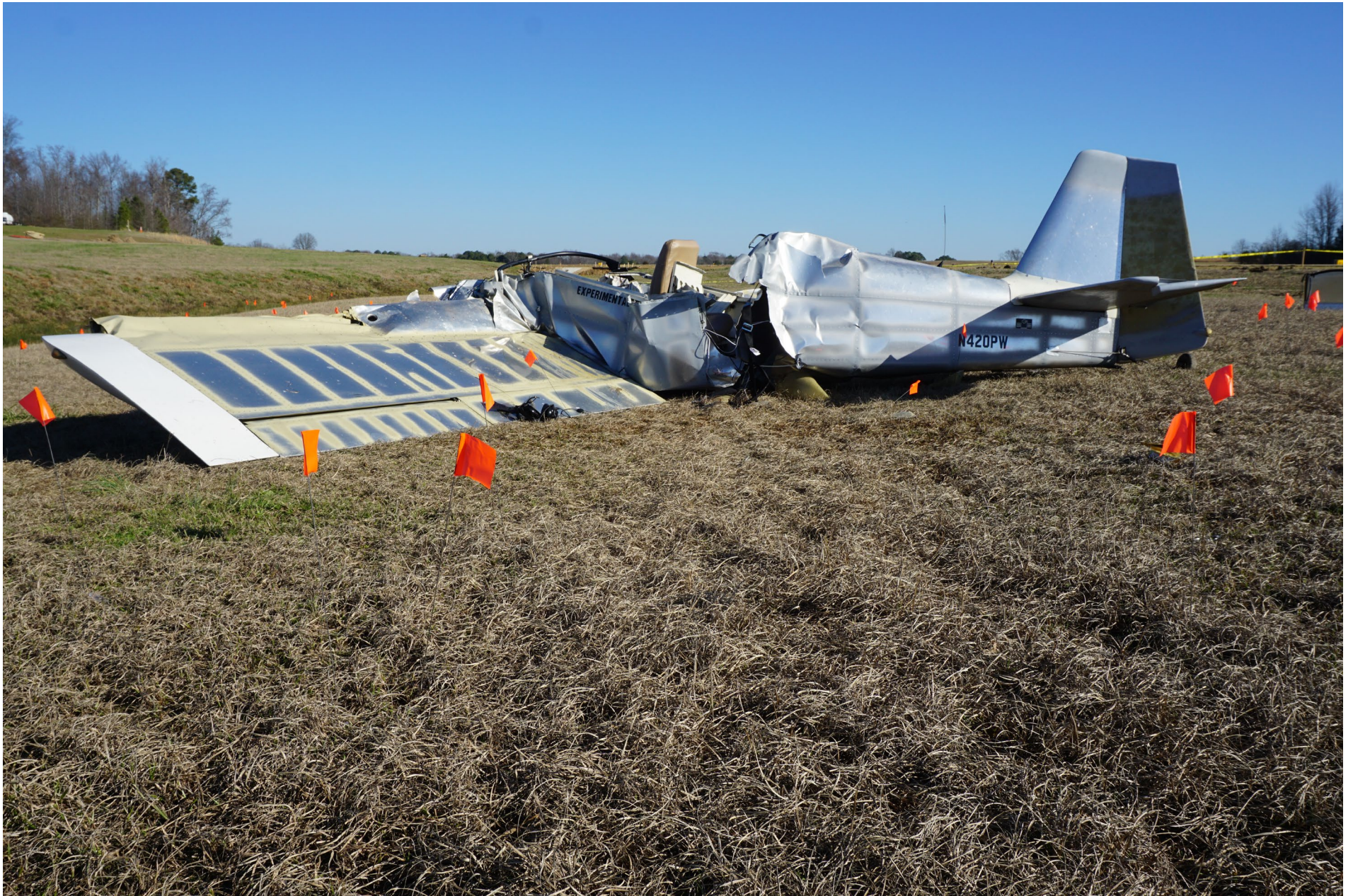
Photo 4 – Left side view of airplane showing crush damage.
