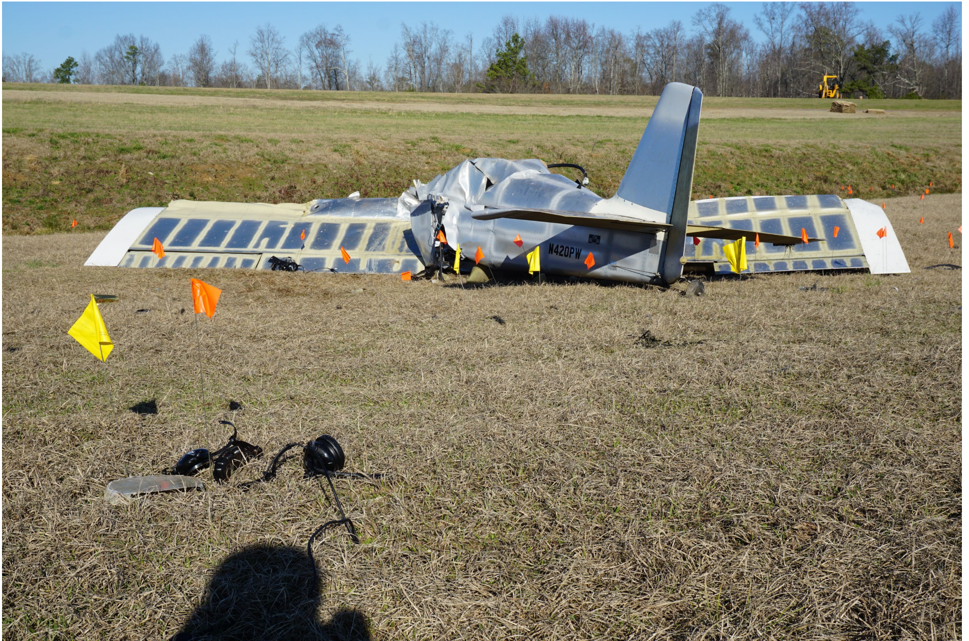
Photo 1 – Aft view of airplane showing fuselage damage.
