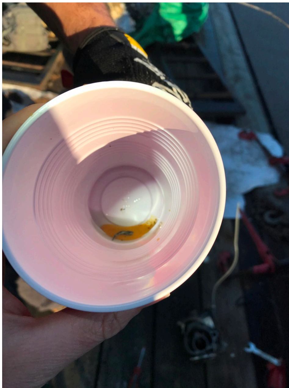
Photo 11 – Rust Colored Fluid drained from Carburetor Bowl
