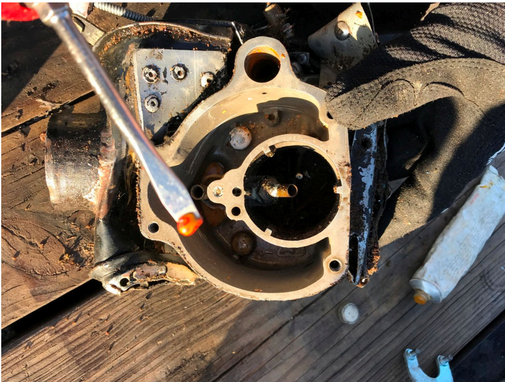
Photo 10 –Water Finding Paste Tests Positive (paste turns pink) in Carburetor Bowl
