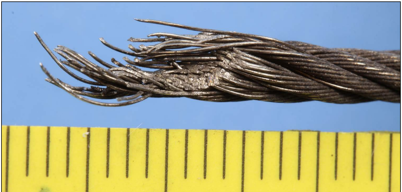
Figure 2. Separated end of the longer cable piece.
