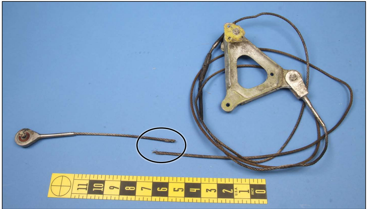
Figure 1. Overall view of the submitted control cable assembly. The location of the cable separation is indicated by an ellipse.
