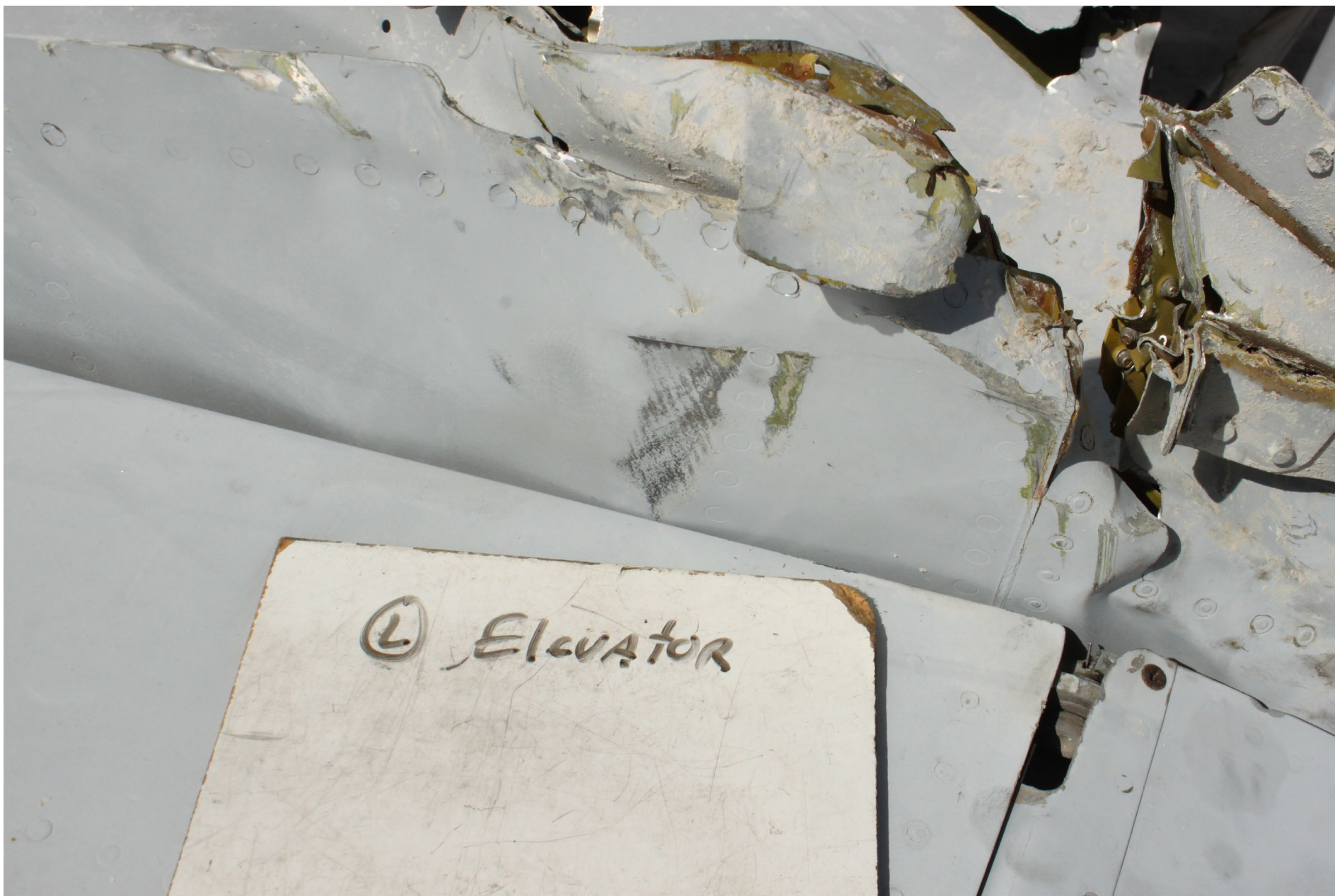
Photo 11 - NTSB Digital Photograph. View Showing the Static Imprint of the Inboard End of the Left Elevator Against the Adjacent Aft Empennage Skin.
