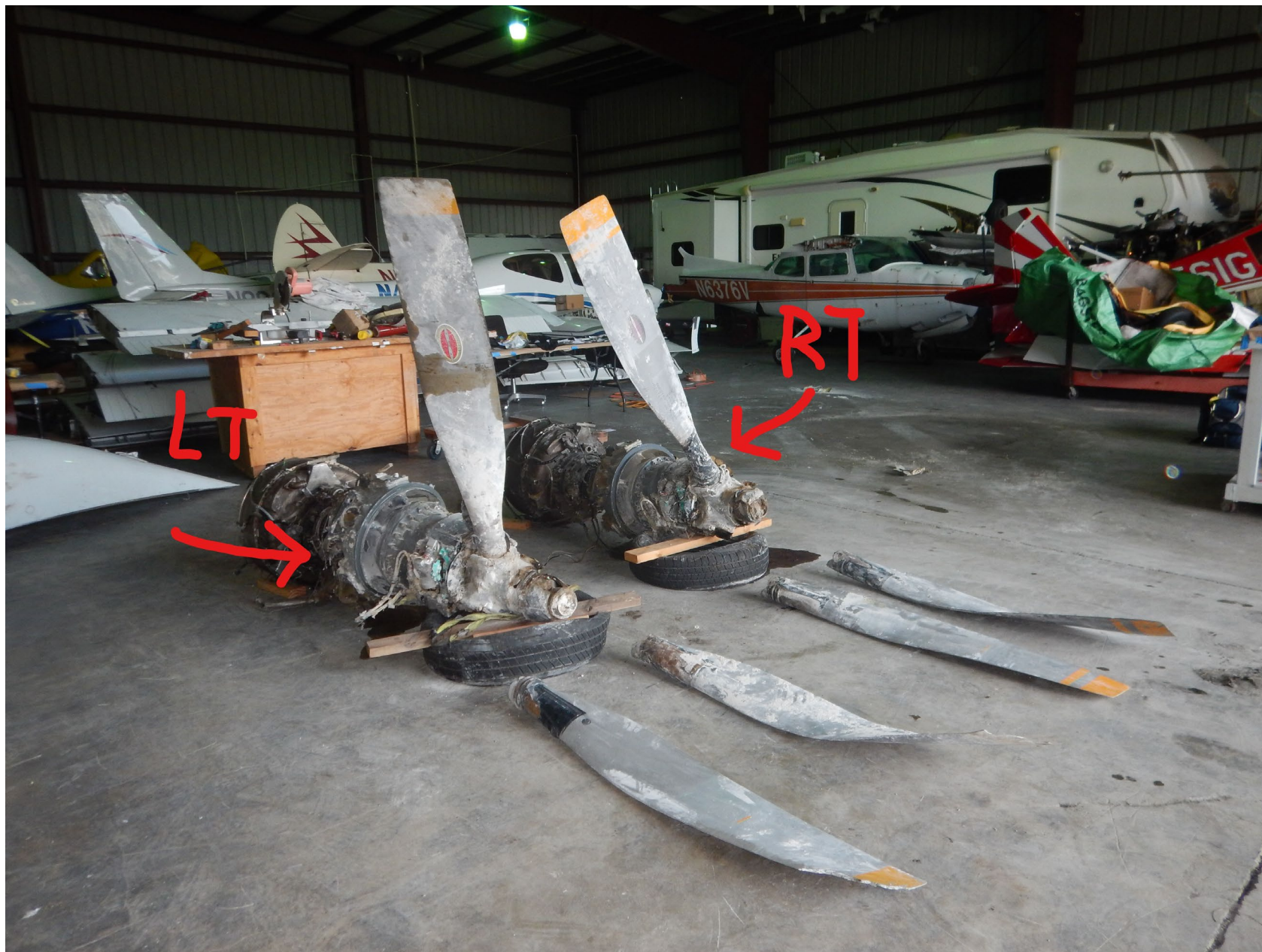
Photo 12 - NTSB Digital Photograph. Annotated Photograph Showing each Engine, Propeller, and Separated Propeller Blades.
