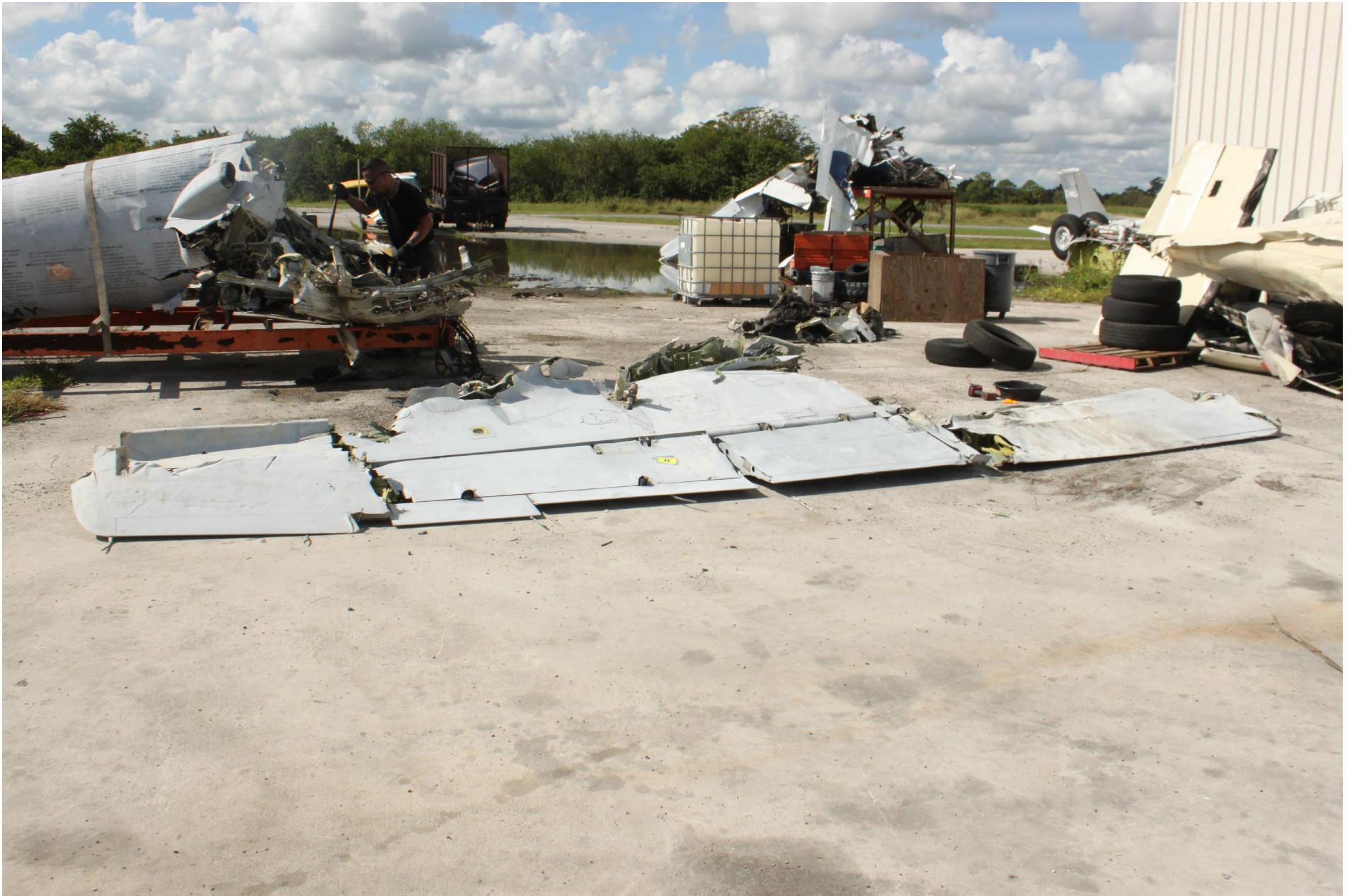
Photo 10 - NTSB Digital Photograph. View of the Reconstruction of the Right Wing.
