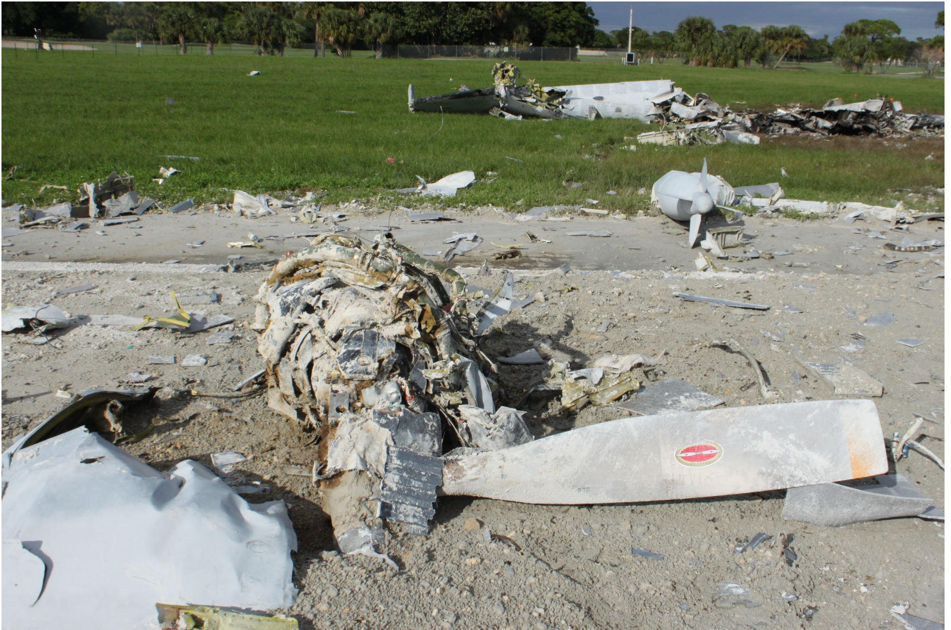
Photo 3 - NTSB Digital Photograph. View of One Propeller Blade of the Left Propeller and Left Engine on Initial Impact Site. Also note, nearby wreckage.
