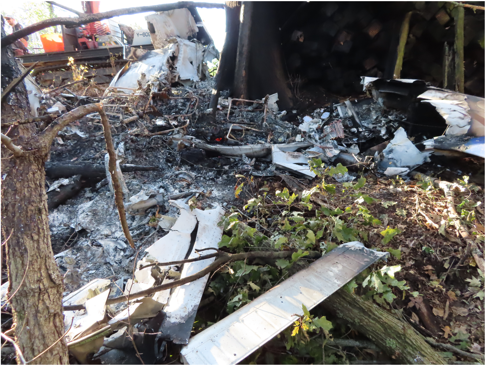
Photo 2 – View of Cockpit and Cabin Area as Found (Piper)
