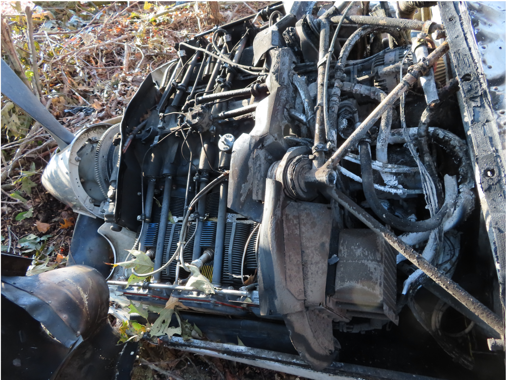
Photo 3 – View of Engine Un-cowled (Piper)
