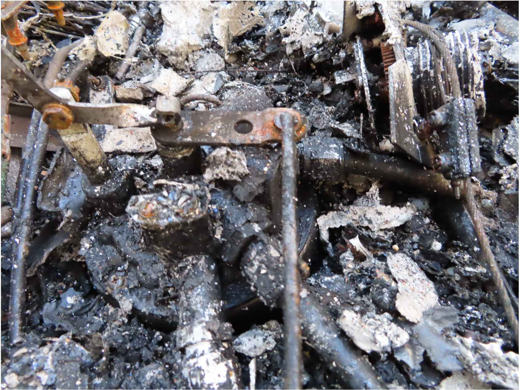
Photo 4 – View of Fuel Selector Valve as Found (Piper)
