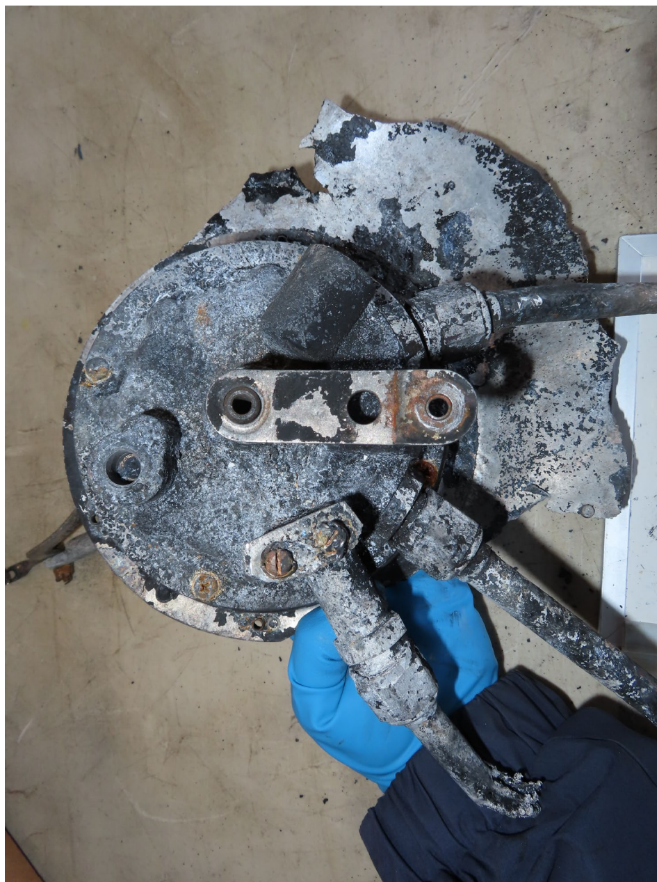
Photo 5 - View of Fuel Selector Valve after Recovery (Piper)
