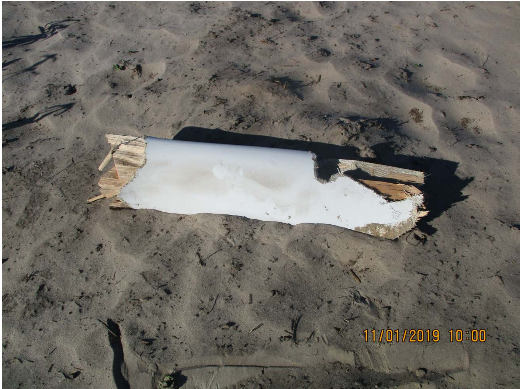
Photo 7 – propeller blade, powerline impression
