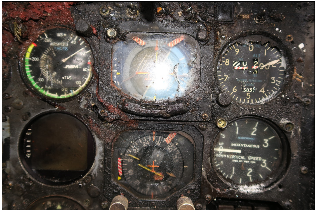
Photo 10: View of the primary flight instruments located on the left side of the cockpit.
