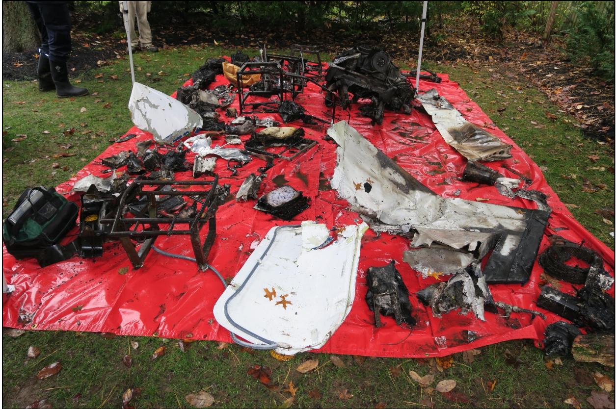
Photo 9: Overview of airframe fragments located in debris
