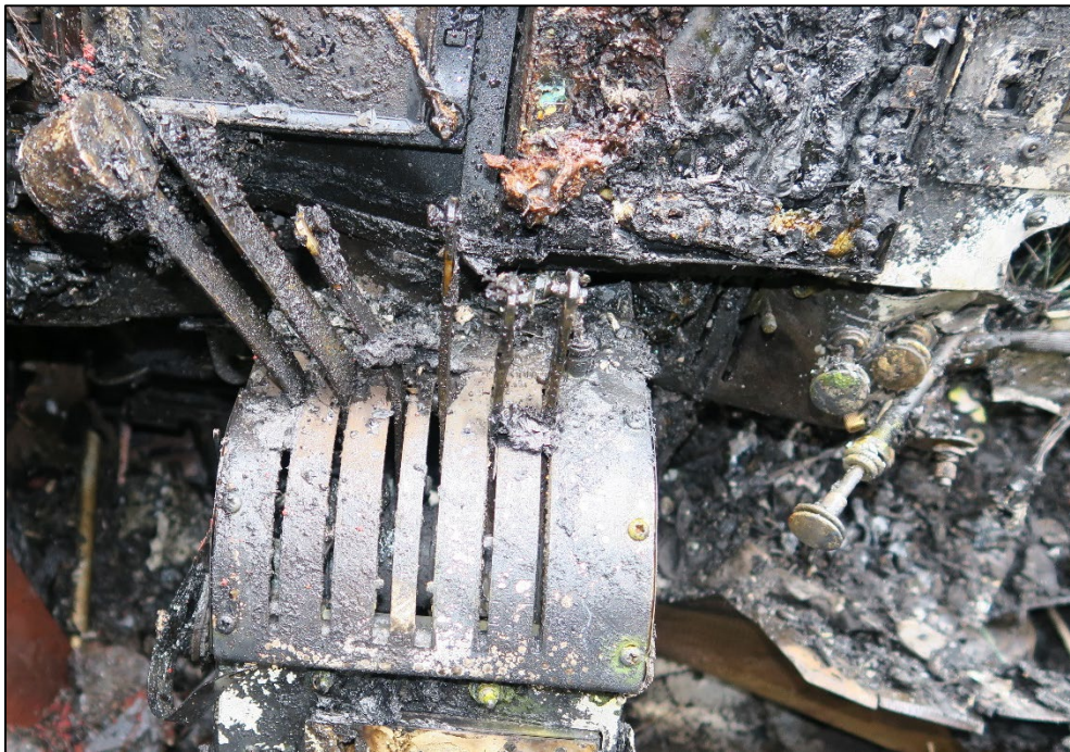
Photo 7: The throttle, mixture, and propeller control quadrant.
