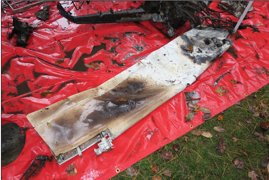
Photo 8: View of fragmented flight control surface
