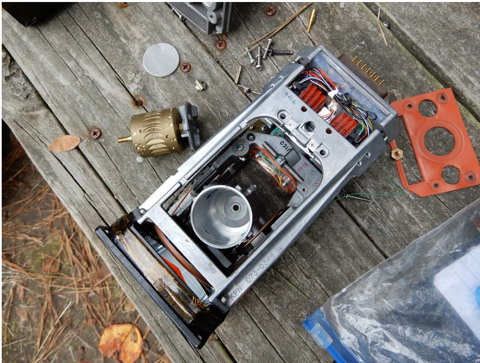
Photo 11 – Attitude Gyro (NTSB Photo)
