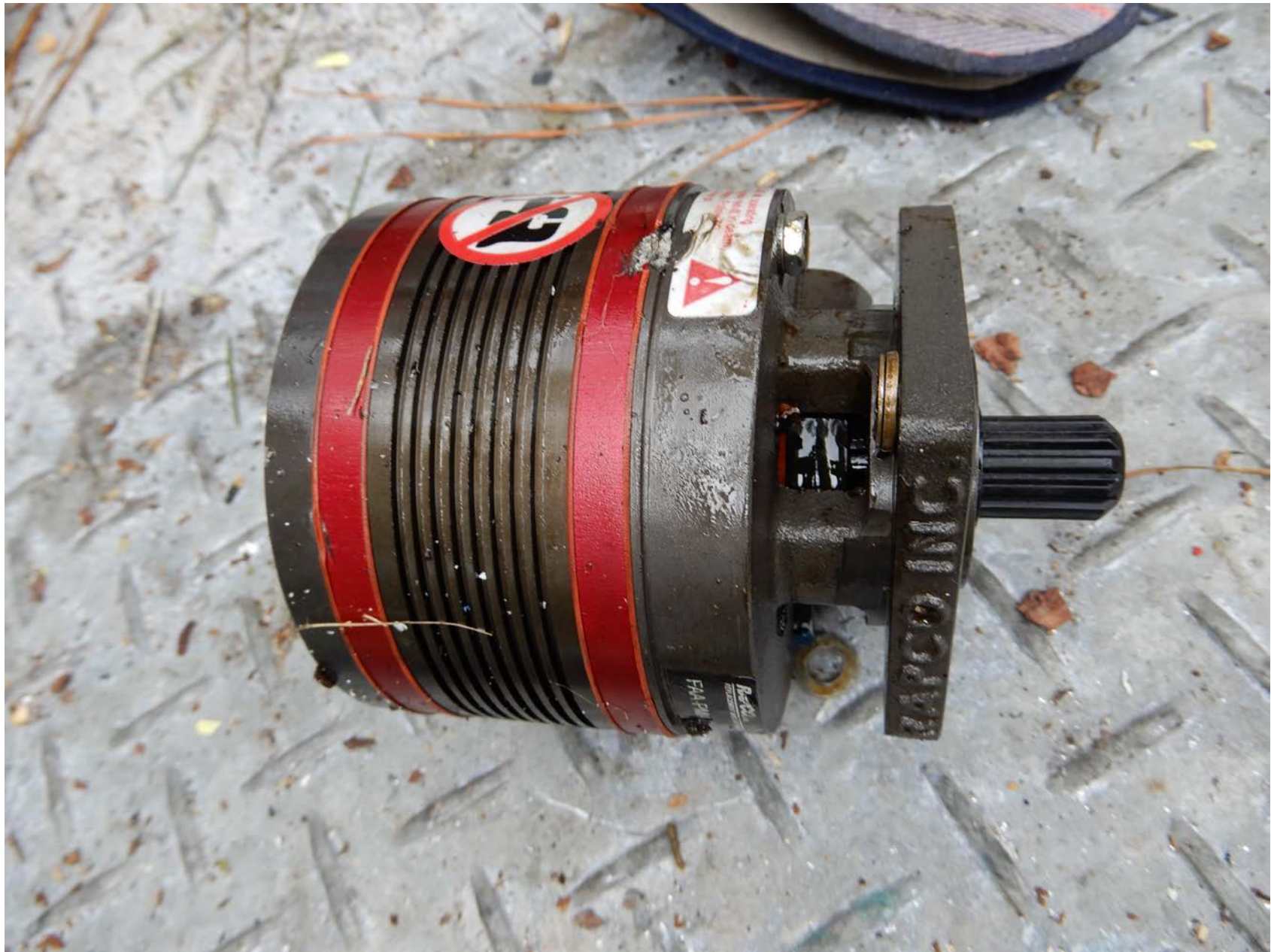
Photo 10 – Vacuum Pump (NTSB Photo)
