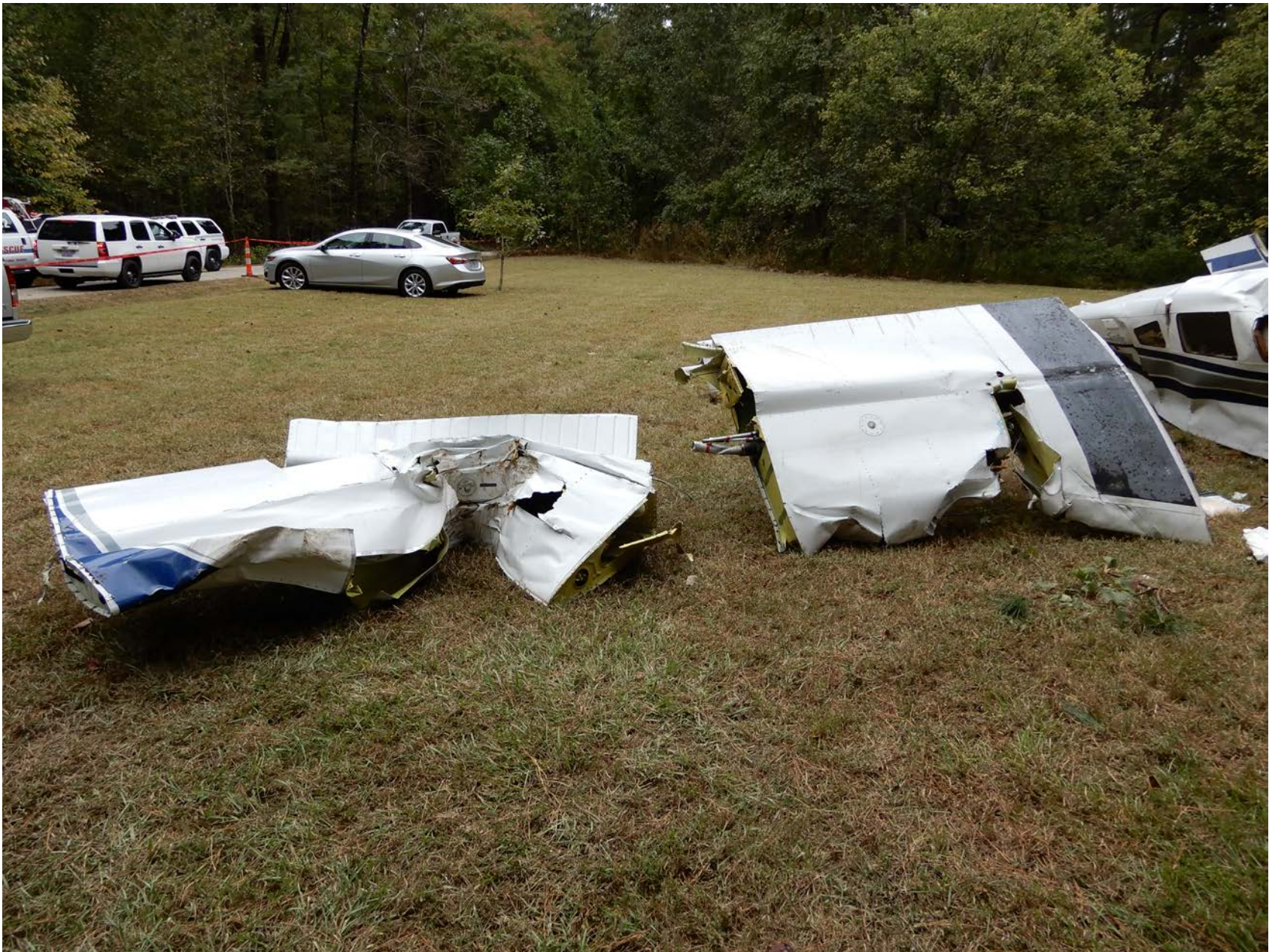
Photo 8 – Right Wing (NTSB Photo)
