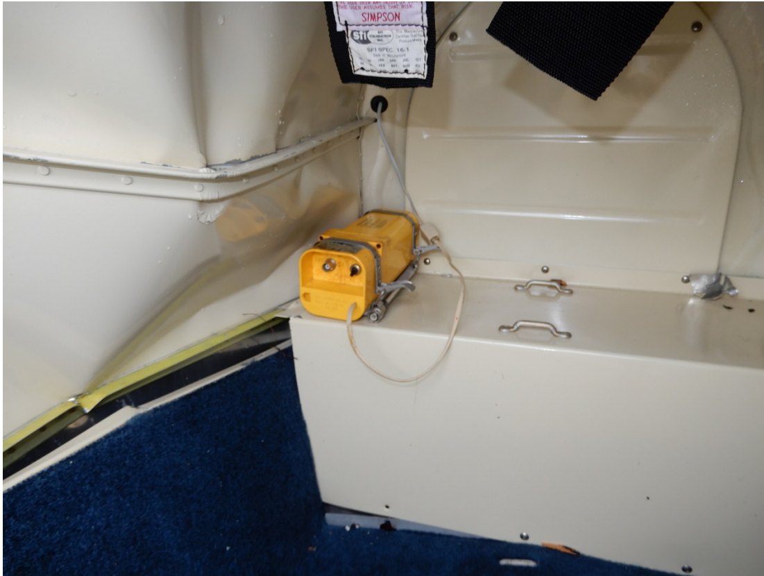
Photo 8: Emergency locator transmitter as found (NTSB Photo)
