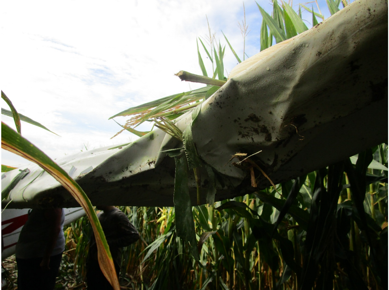
Photograph 3 3 – Accident airplane – left wing substantial damage.
