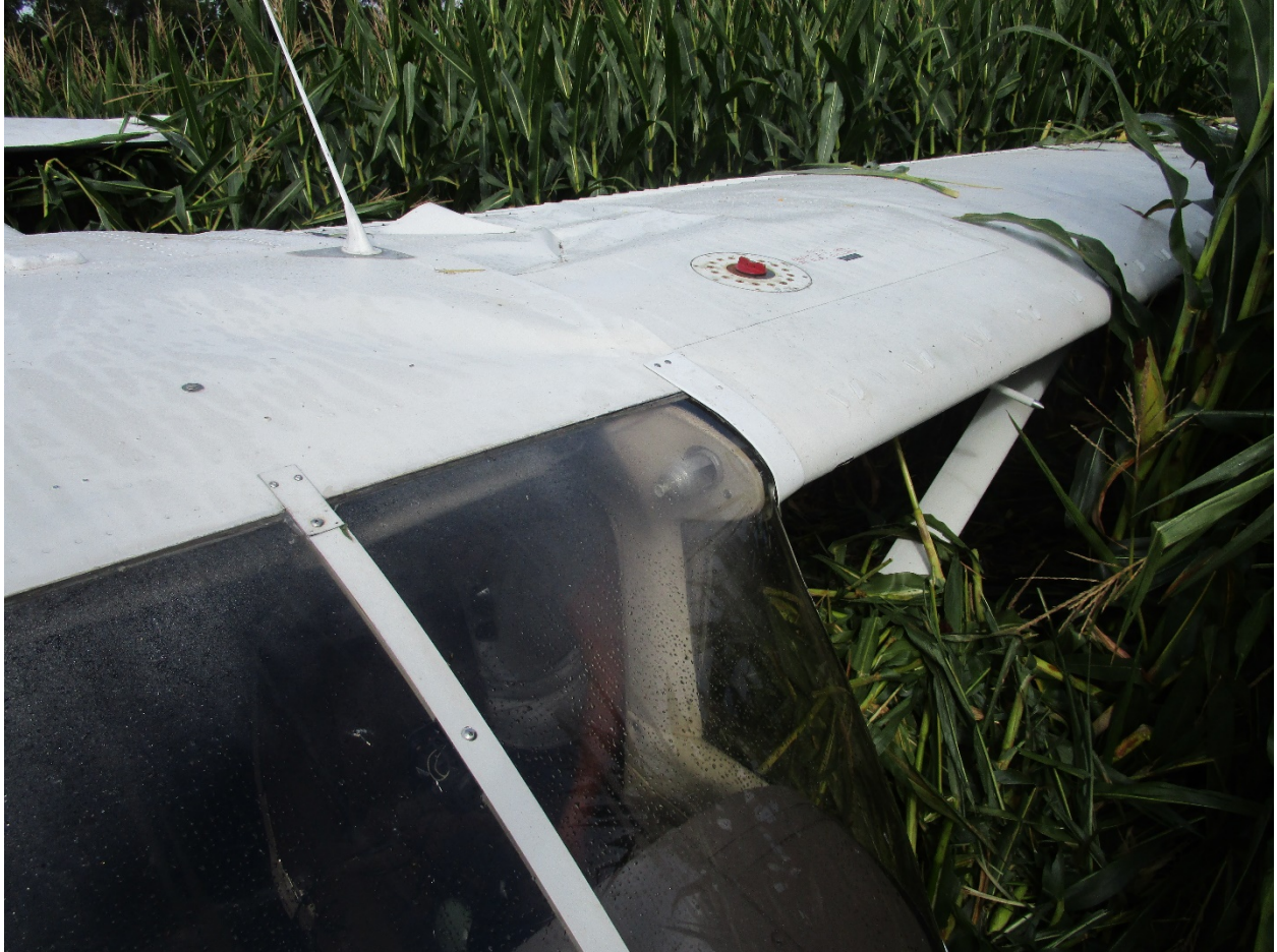
Photograph 2 2 – Accident airplane – left wing substantial damage.
