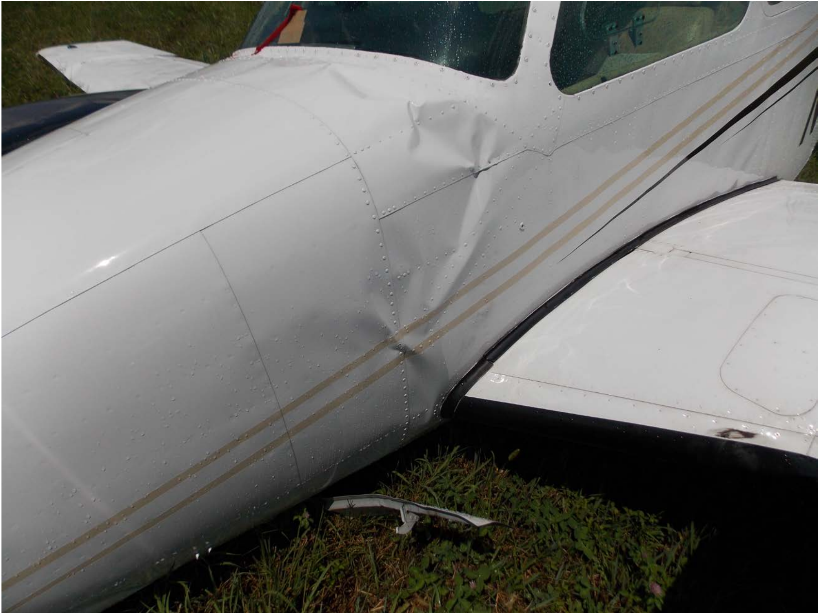
Photo 2 – View of Fuselage Damage (FAA)
