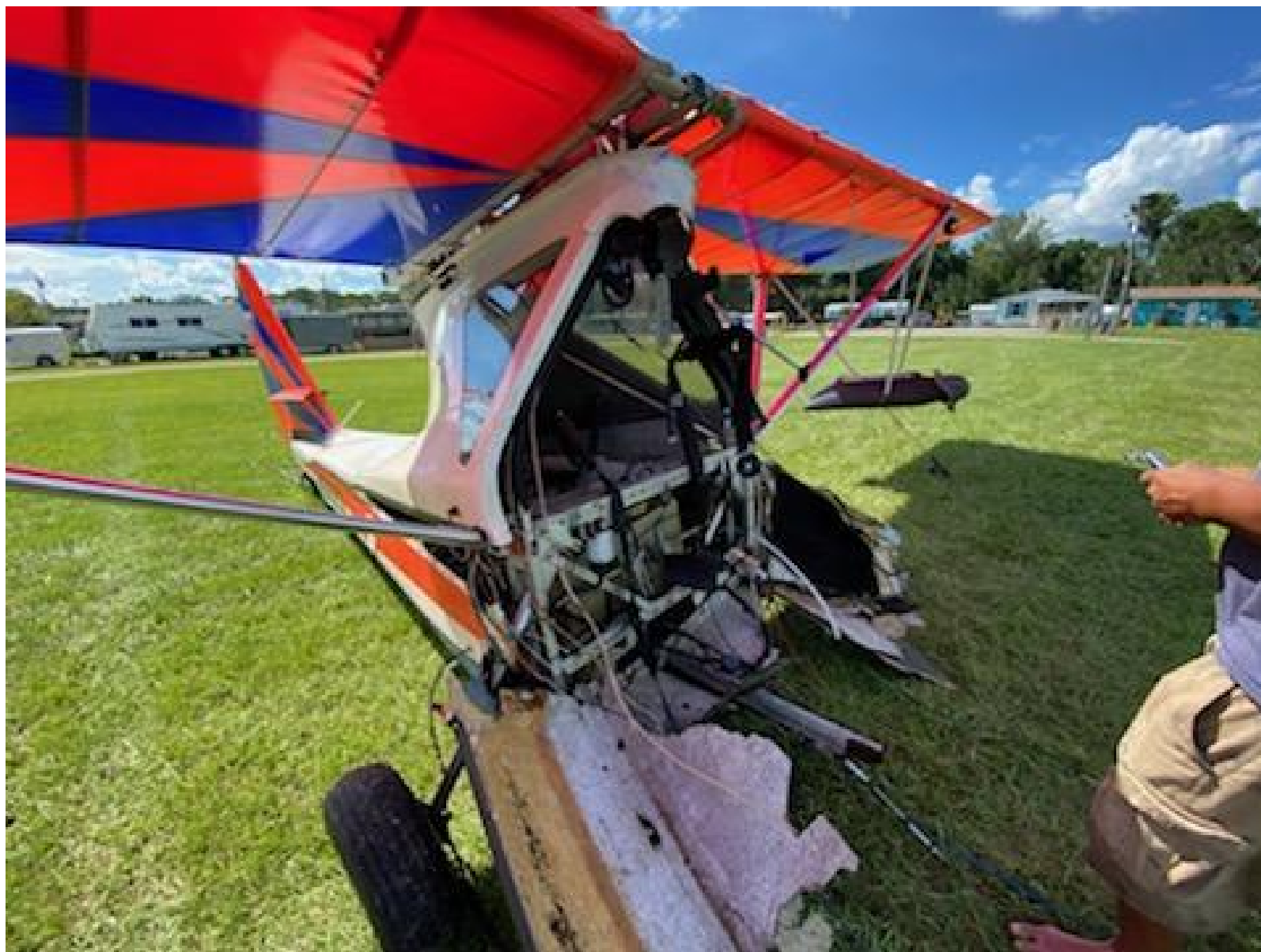
Photo 1 – View of Airplane Damage After Water Recovery. (Courtesy of Pilot/Owner)
