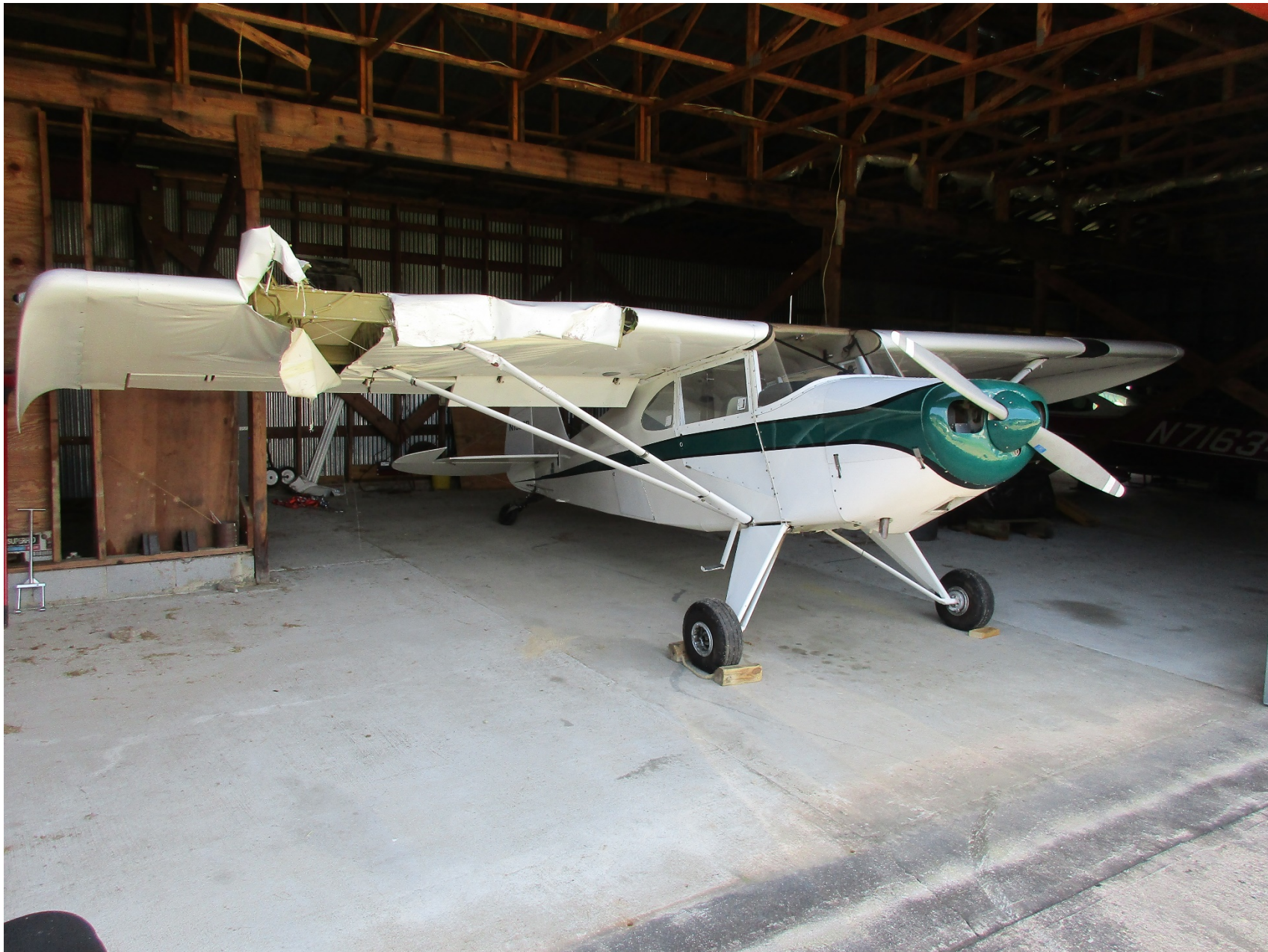
Photo 1 – front right quartering wing damage.
