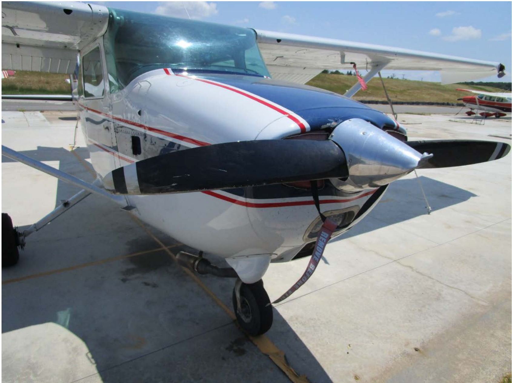
Photo 1 – Propeller, Propeller Spinner, and Left Wing Tip Damage - Courtesy of Harford Air Services
