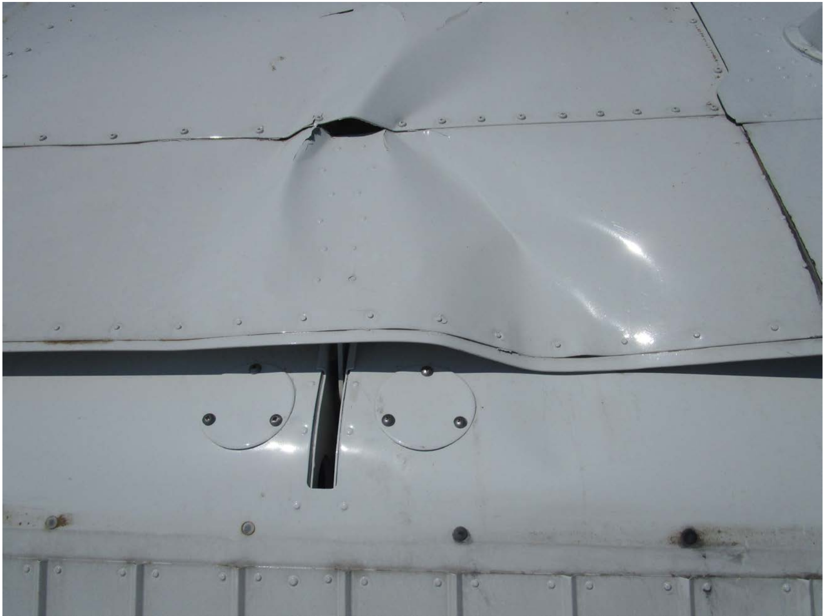
Photo 3 – Top View of Upper Left Wing Damage – Courtesy of Harford Air Services
