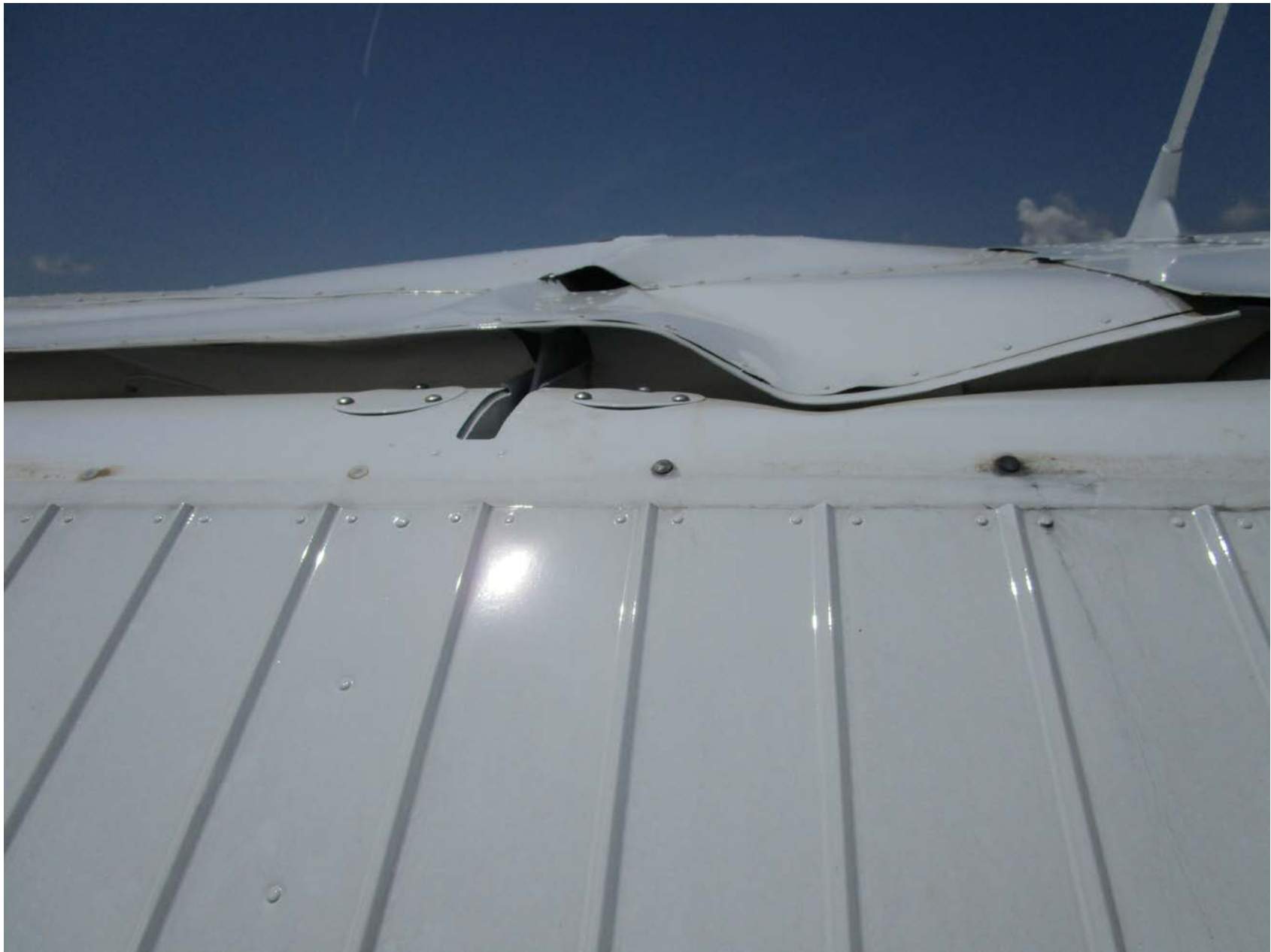
Photo 4 – Aft View of Upper Left Wing Damage – Courtesy of Harford Air Services
