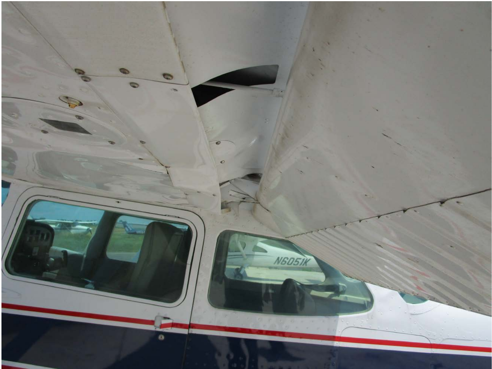
Photo 2 – Lower Left Wing Damage - Courtesy of Harford Air Services)
