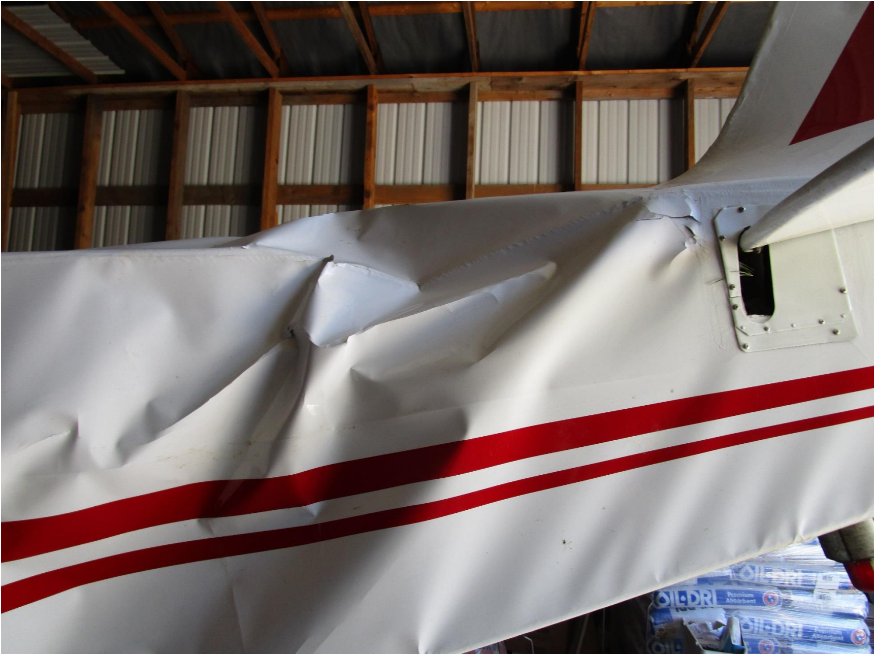
Airplane – View of Fuselage Damage (courtesy FAA)
