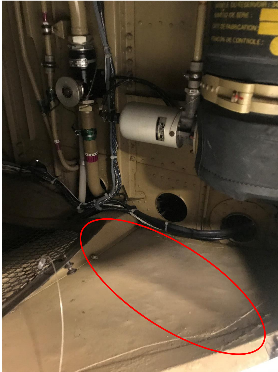
Interior Floor Deformation (courtesy Airbus Helicopters)
