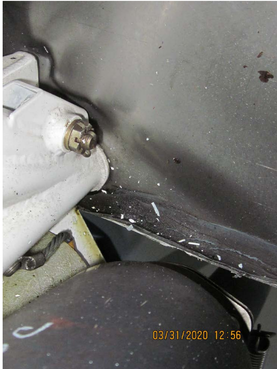
Photo 4 - View of fire wall damage (photo courtesy of the FAA).
