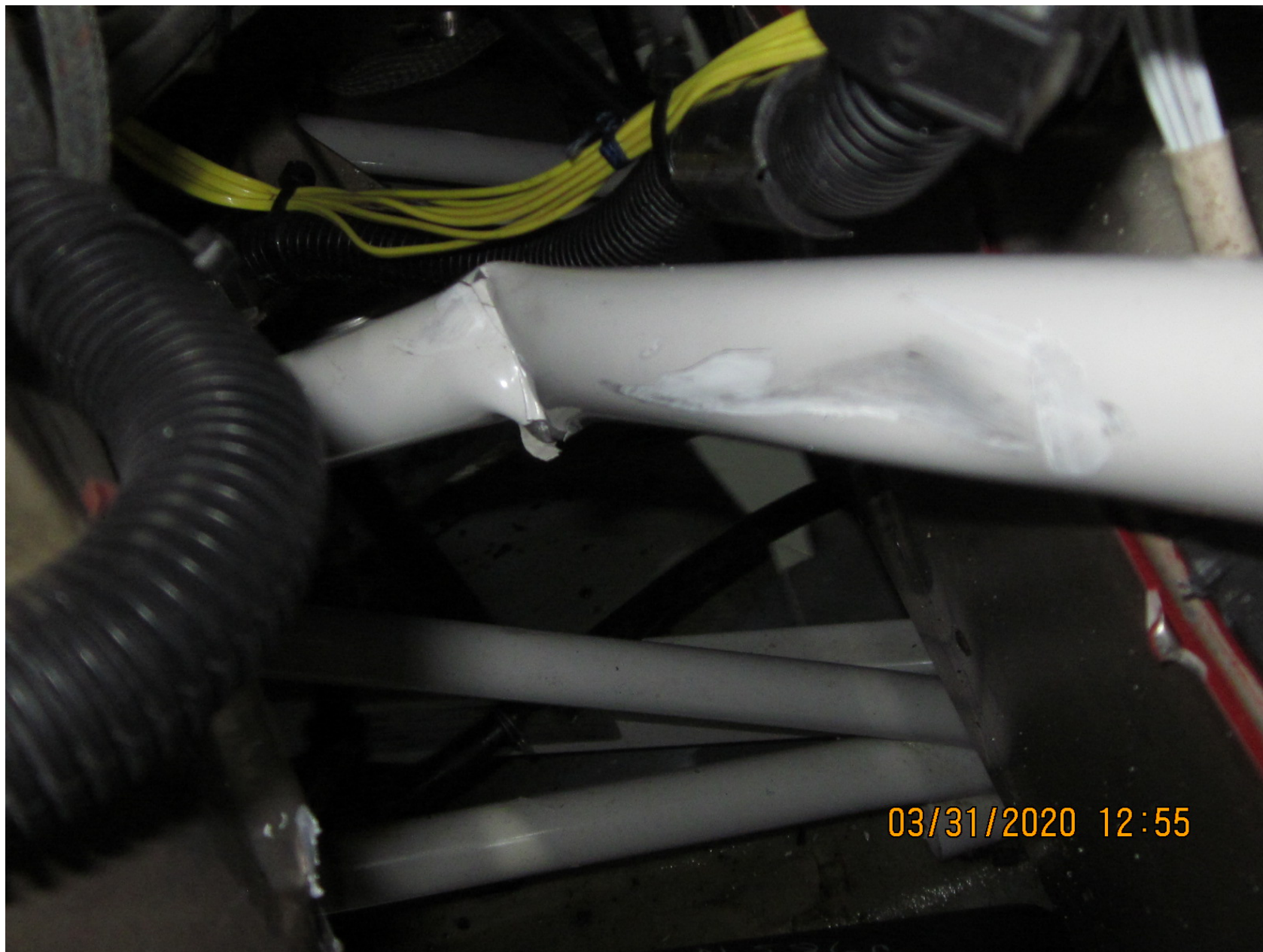
Photo 3 - View of engine mount damage (photo courtesy of the FAA).
