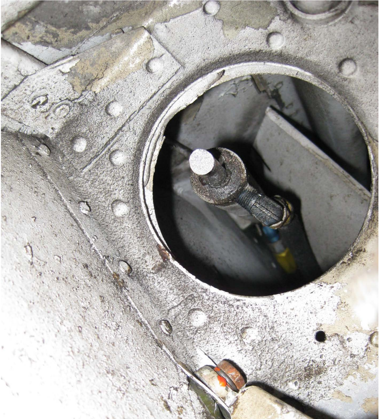
Photograph 1 - Accident airplane right main gear sheared torque link bolt.
