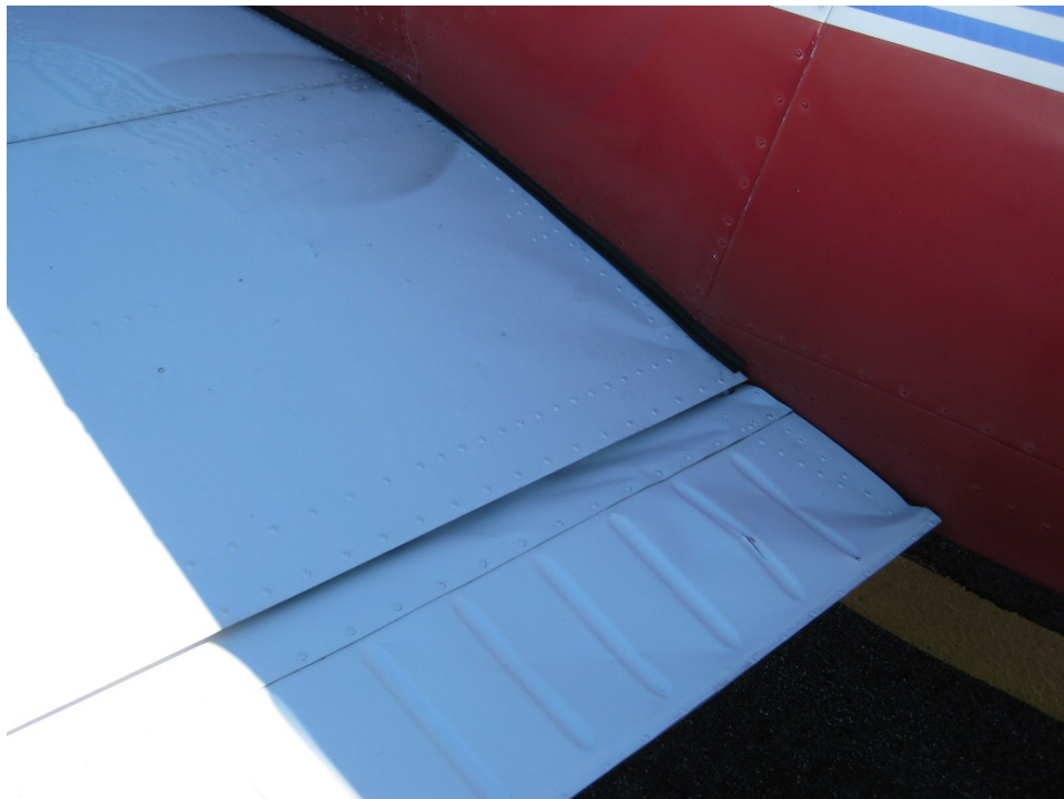
Photograph 3 - Accident airplane left wing damage.
