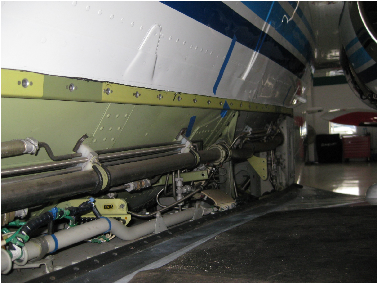
Photo 3 – View of fuselage wrinkling (Courtesy of FAA)
