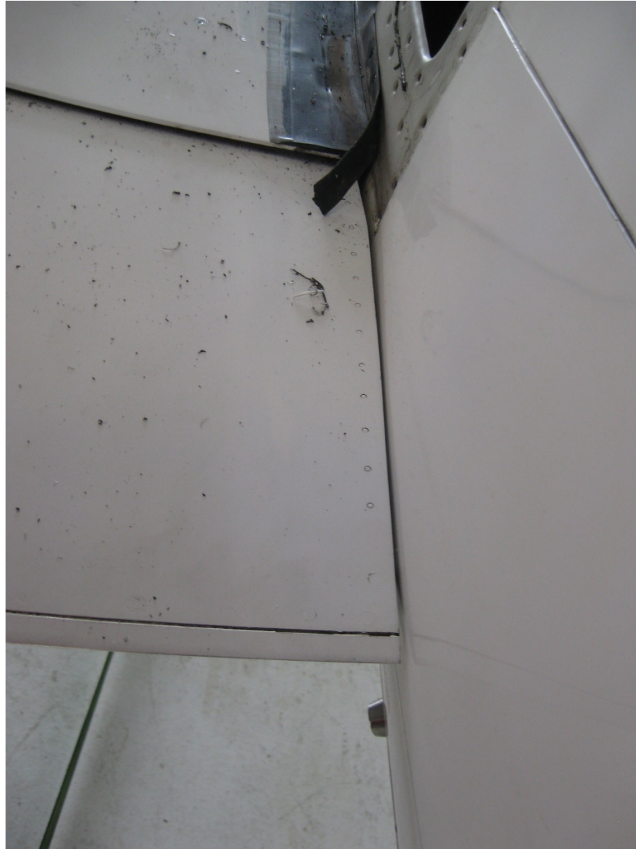
Photo 2 – View of gap between left flap and fuselage (Courtesy of FAA)
