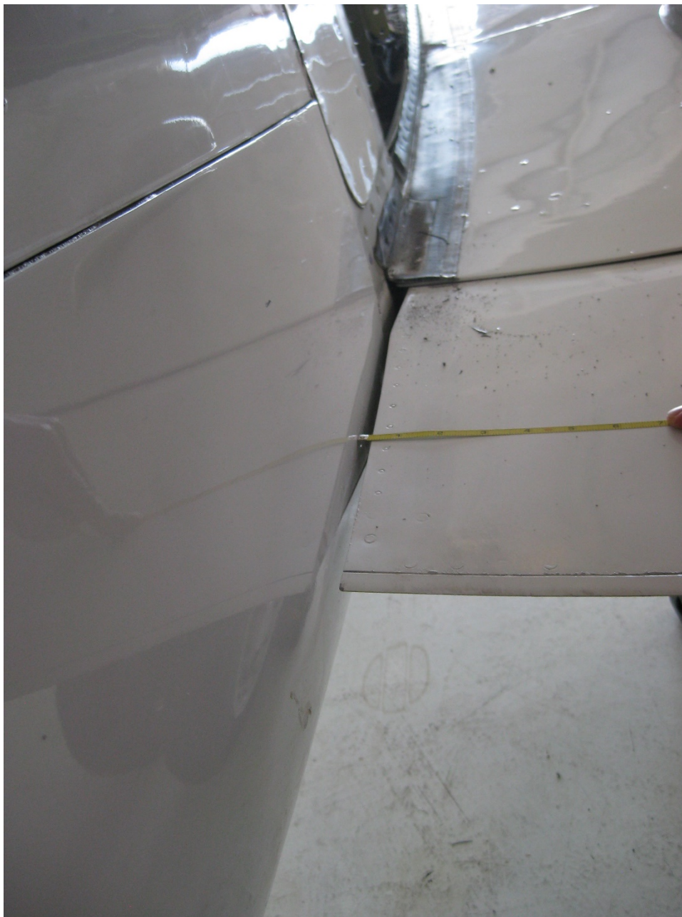
Photo 1 –View of gap between right flap and fuselage (Courtesy of FAA)
