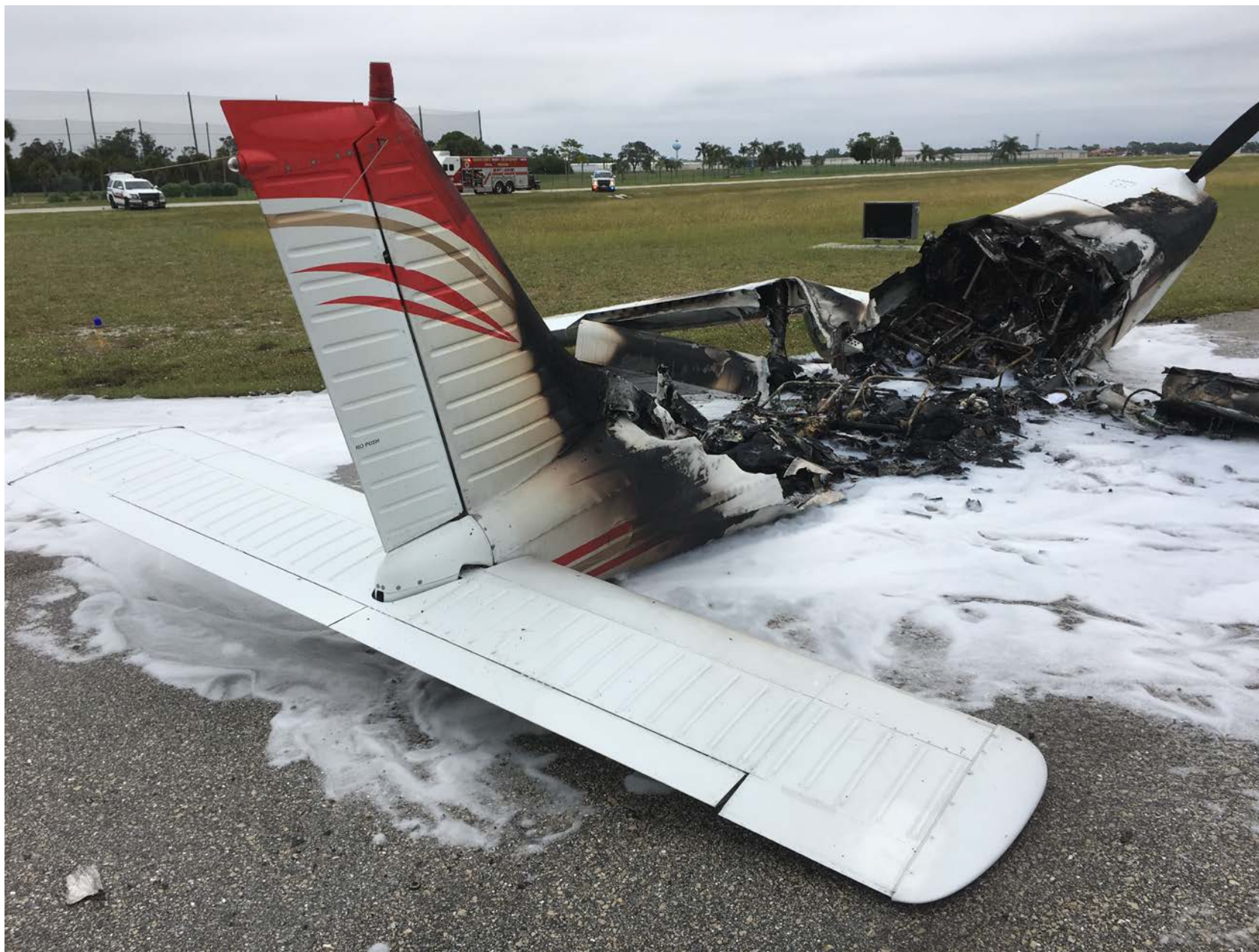
Photo 2 – View of Fire Damage to Cockpit, Cabin, Empennage, and Wings (FAA)
