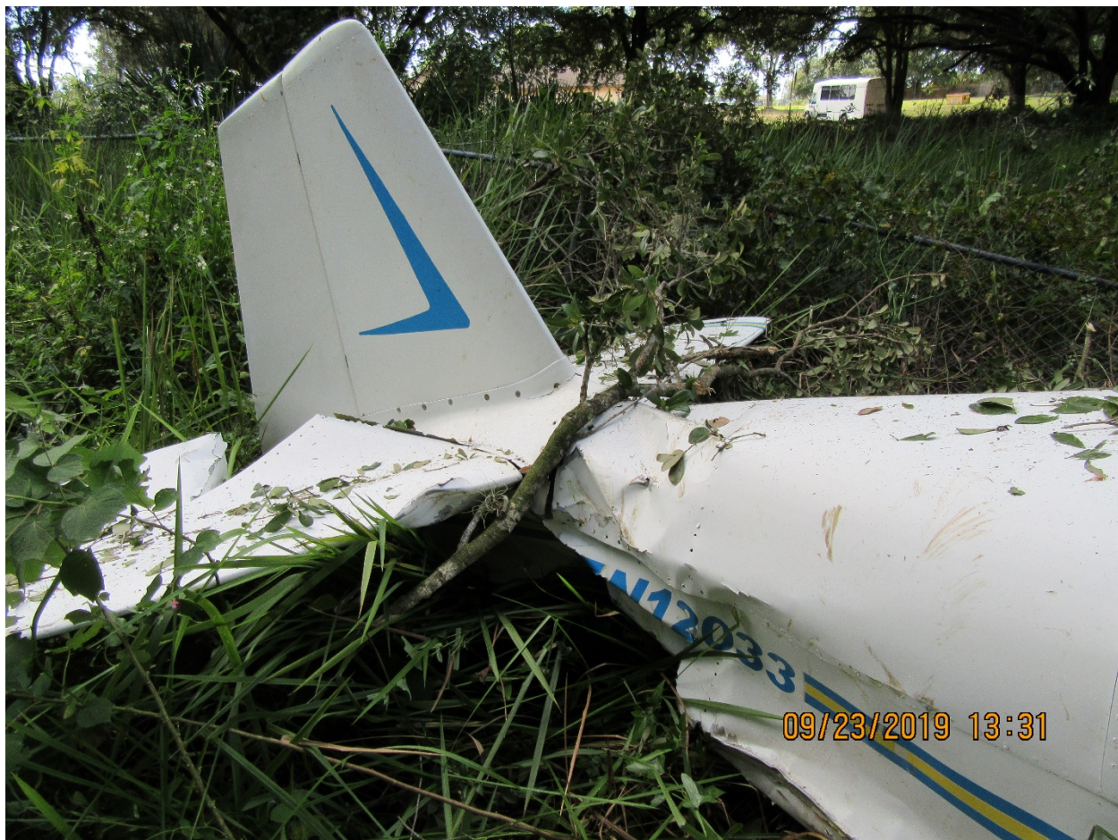
Photograph 4 4 – Accident airplane – tail section damage.
