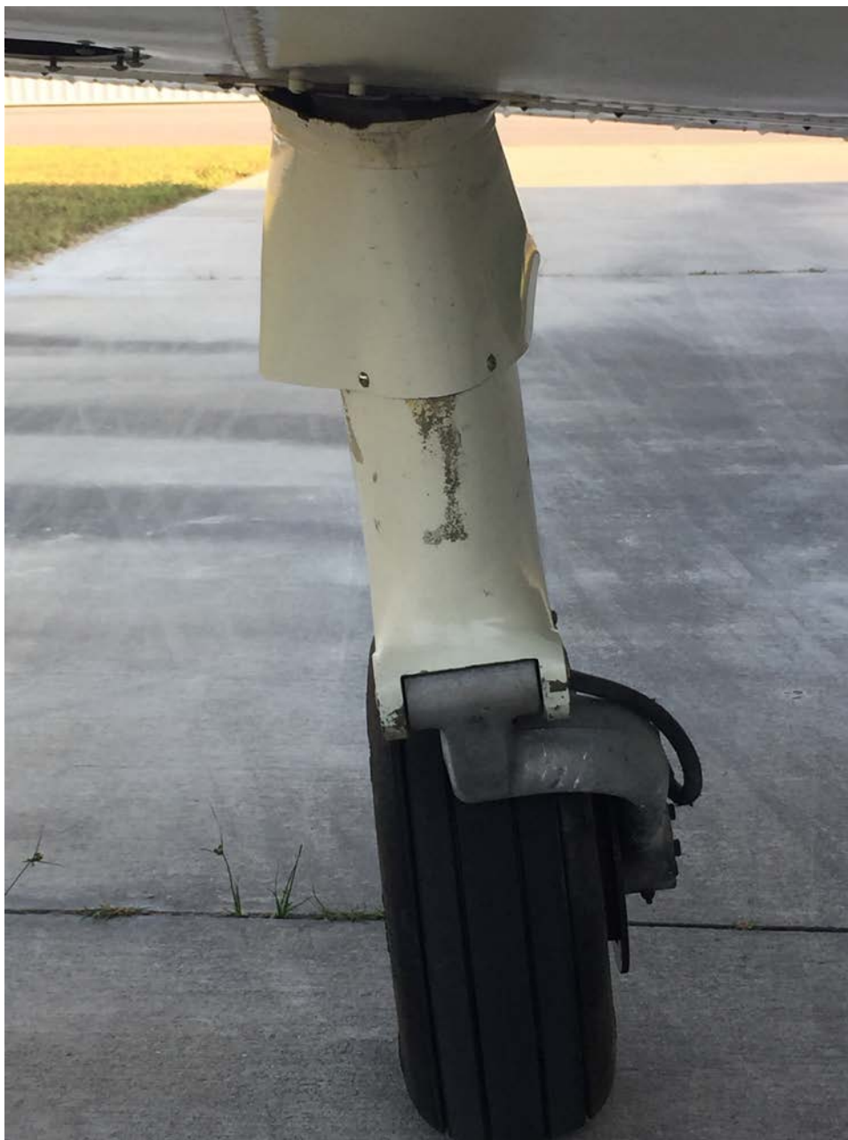
Photo 1 – Forward view of damaged right landing gear. (Courtesy of FAA)
