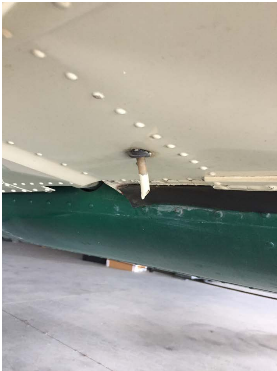
Photo 5 – View of fuel vent that was blocked with debris. (Courtesy of DCAVIATION)
