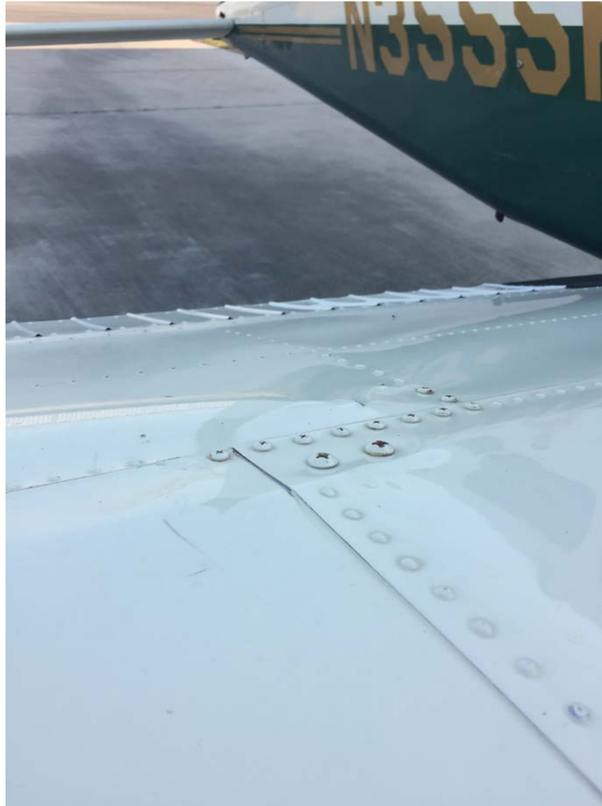
Photo 4 – Right wing looking aft. Note buckling on rivet line. (Courtesy of DCAVIATION)
