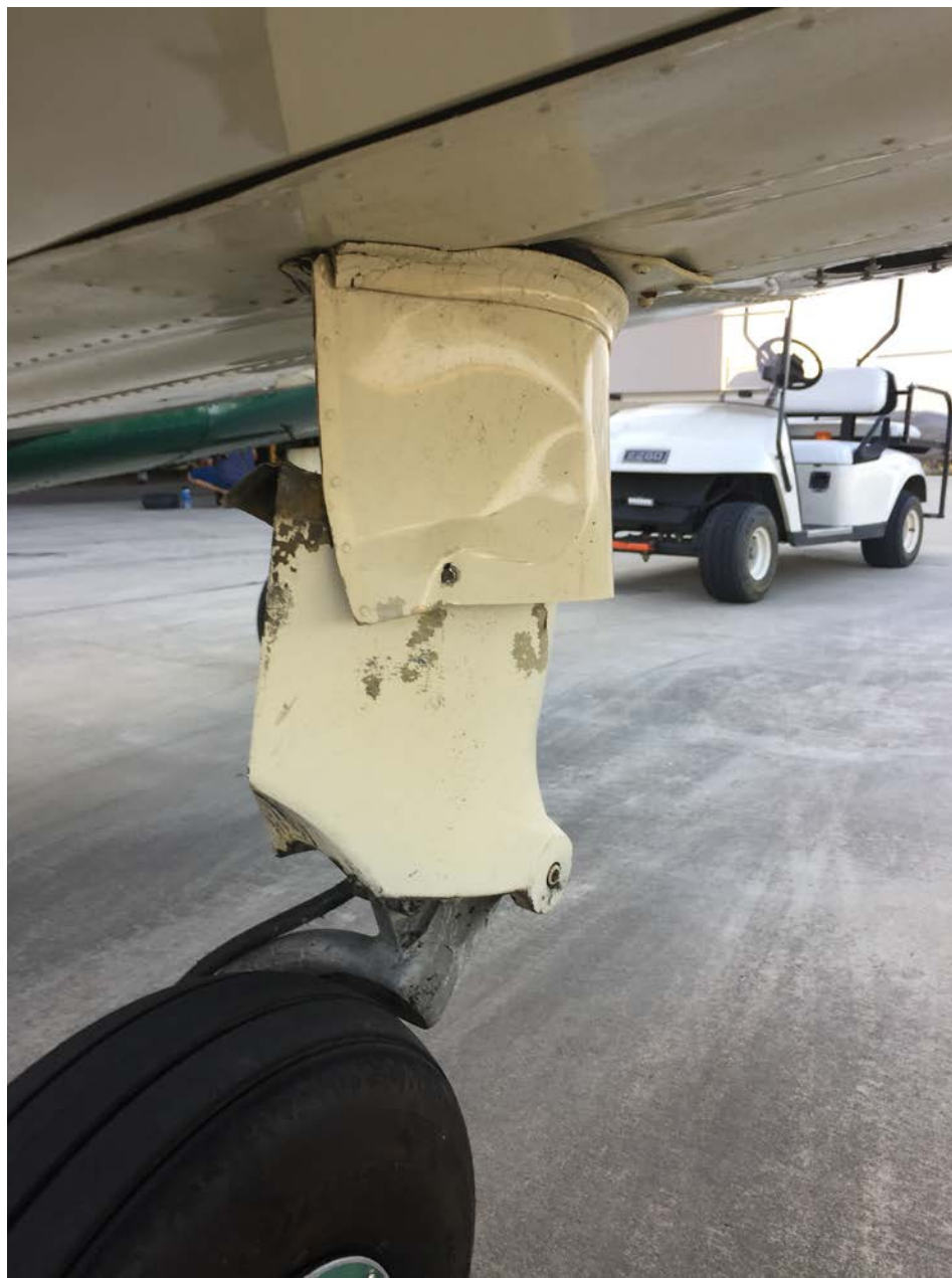
Photo 2 – Damaged right landing gear. (Courtesy of FAA)
