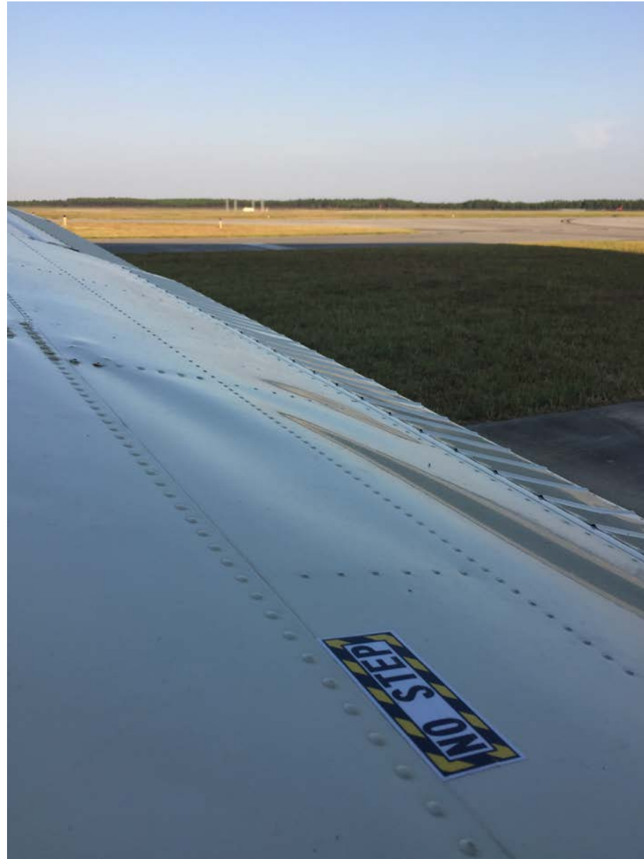
Photo 3 – Top of right wing buckling. (Courtesy of DCAVIATION)
