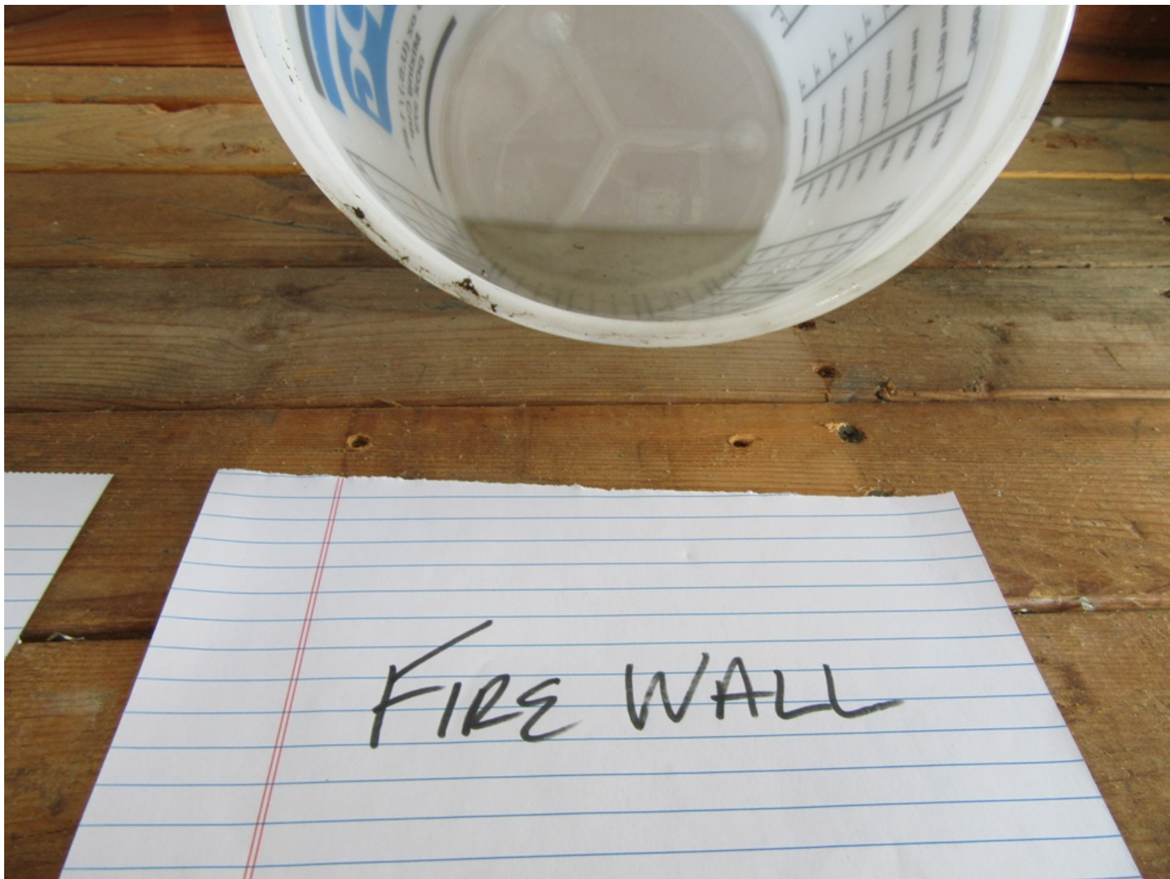
Photo 3 - Fuel Sample From Firewall Sump (Photo Courtesy of FAA)
