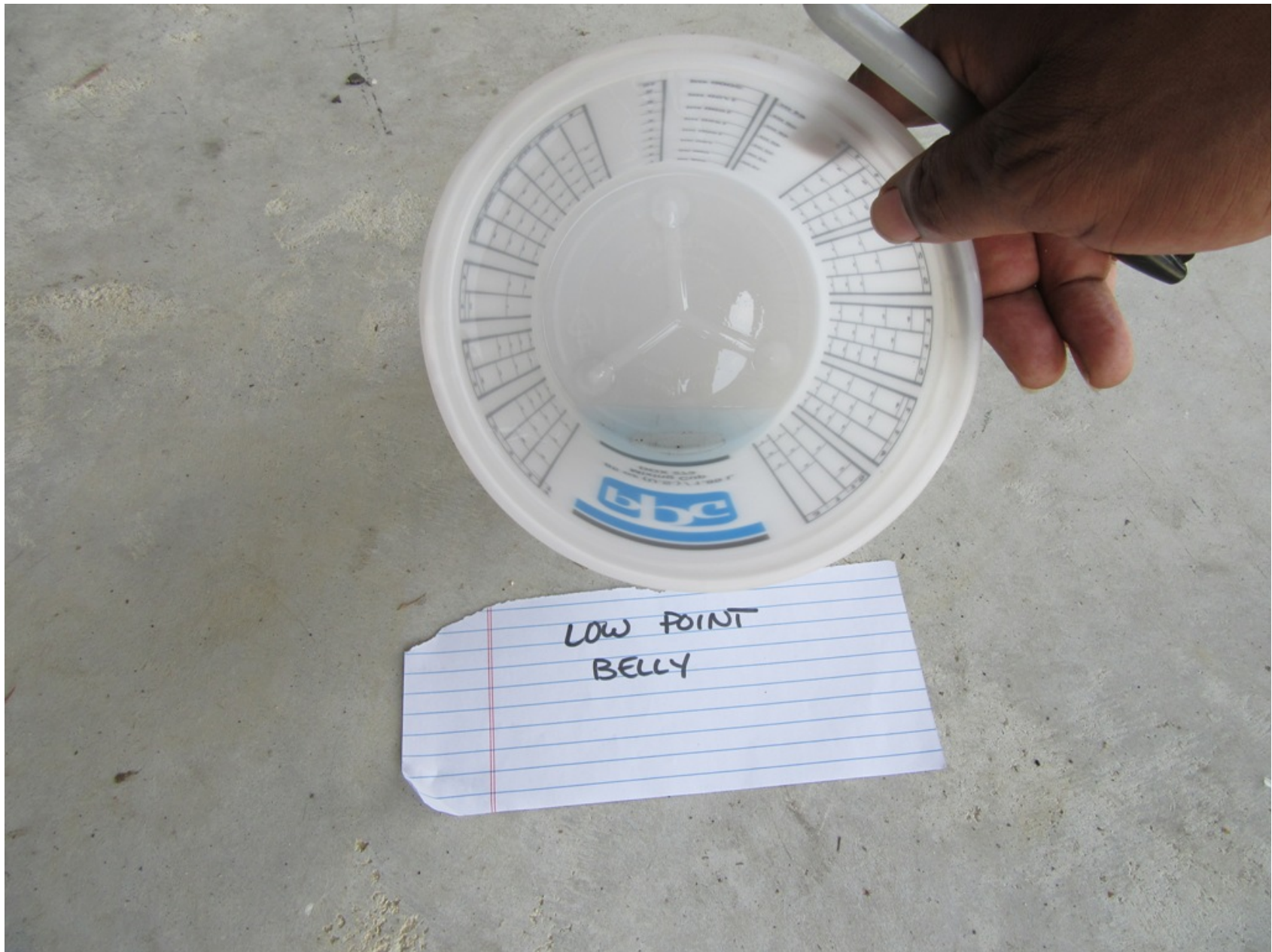
Photo 4 - Fuel Sample From Belly Sump (Photo Courtesy of FAA)
