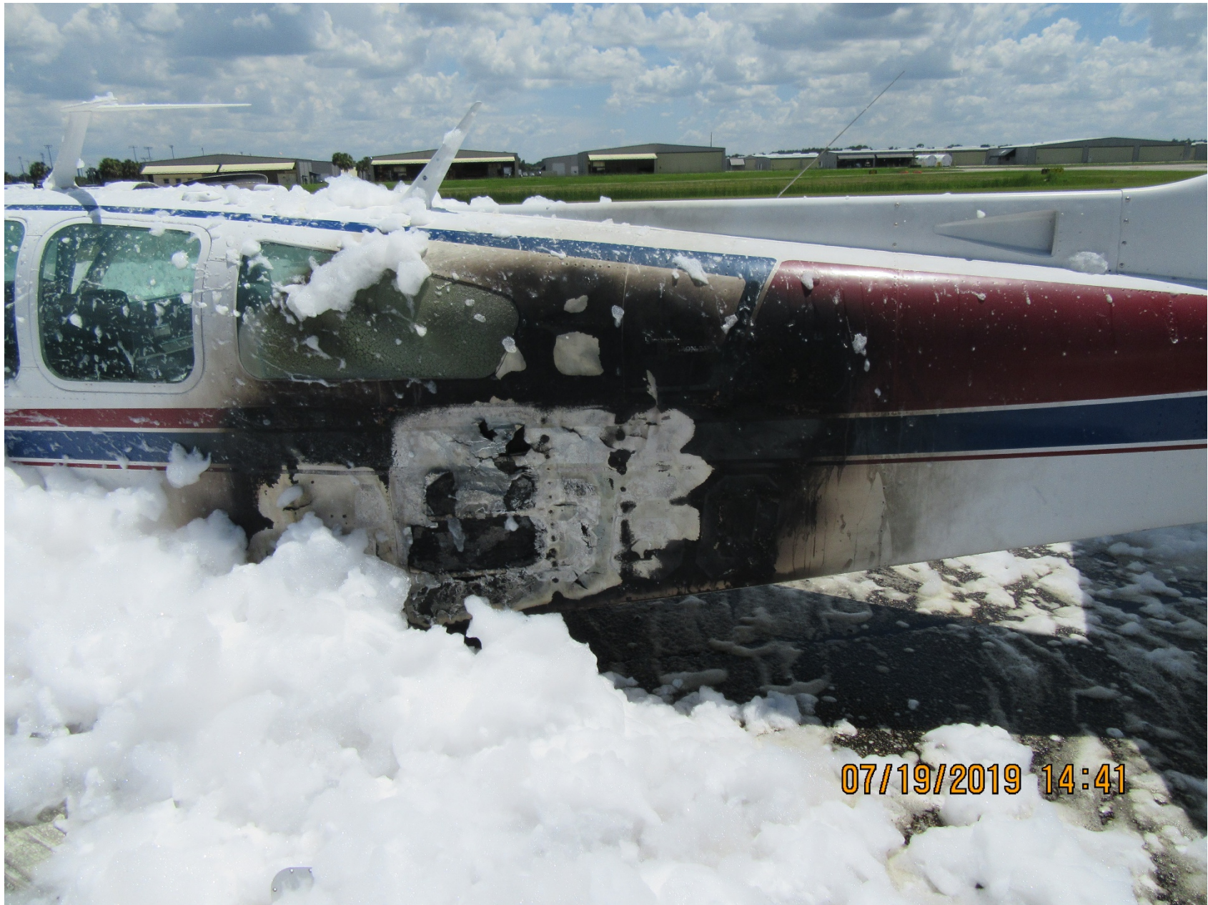
Photo 2 – View of fire damaged left side of airplane
