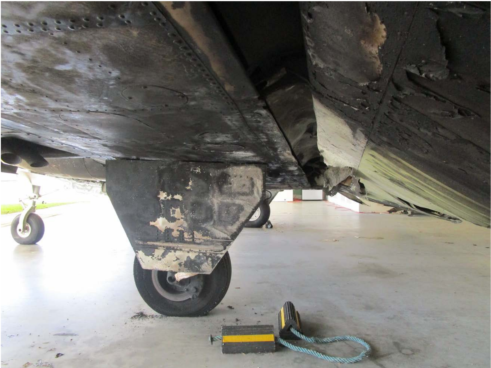
Photo 3 – View of underside of left wing fire damaged and landing gear down and locked
