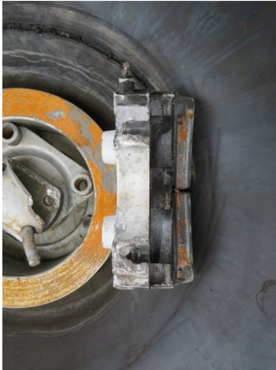
Photo 3 – View of the left brake caliper. (Photo courtesy of the FAA)
