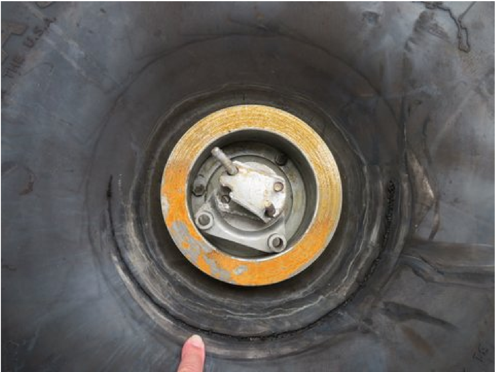
Photo 4 – View of the damage to the left tire. (Photo courtesy of the FAA)
