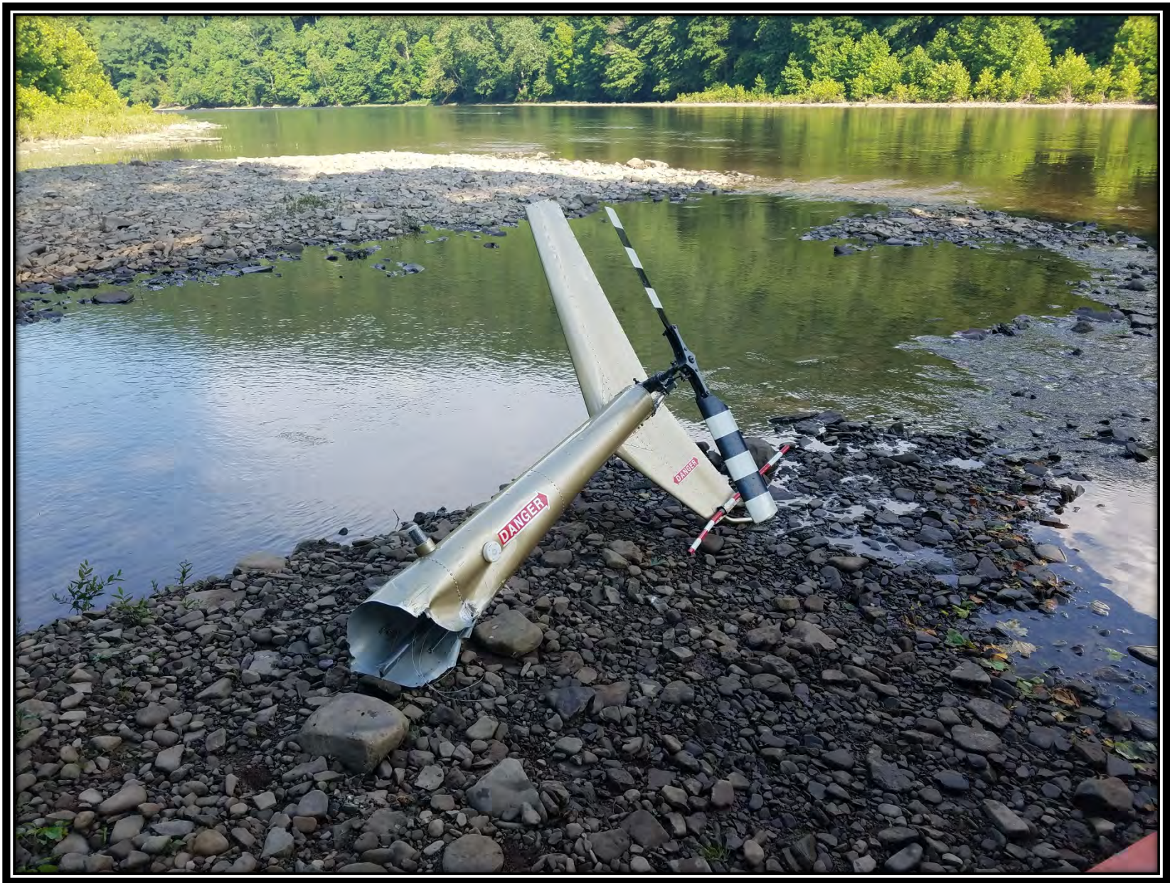
Photo 5 – Separated Tail Boom (Photo Courtesy of FAA)
