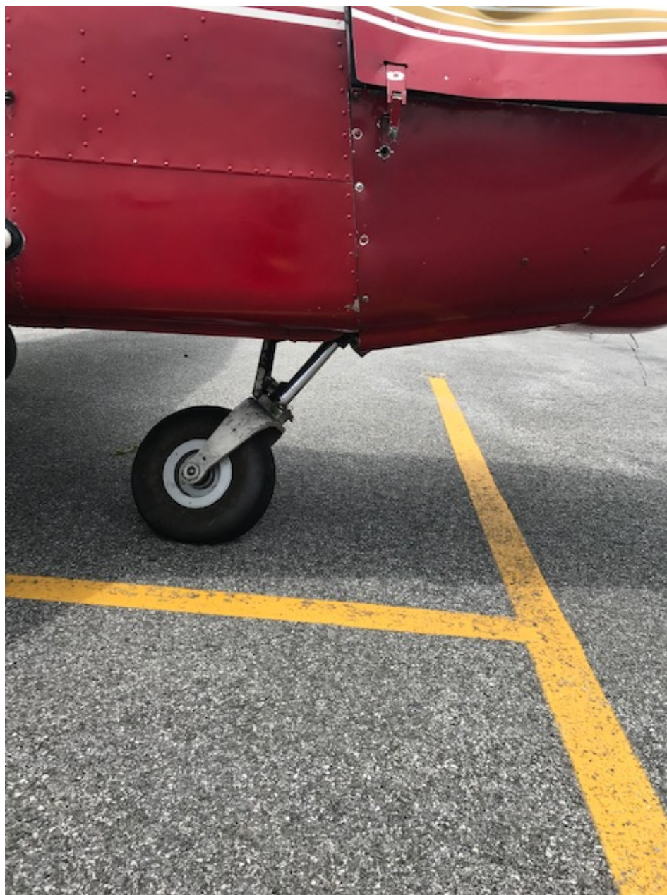
Photo 2 - Courtesy of FAA- side view of airplane showing collapse nose gear and buckled engine cowling.
