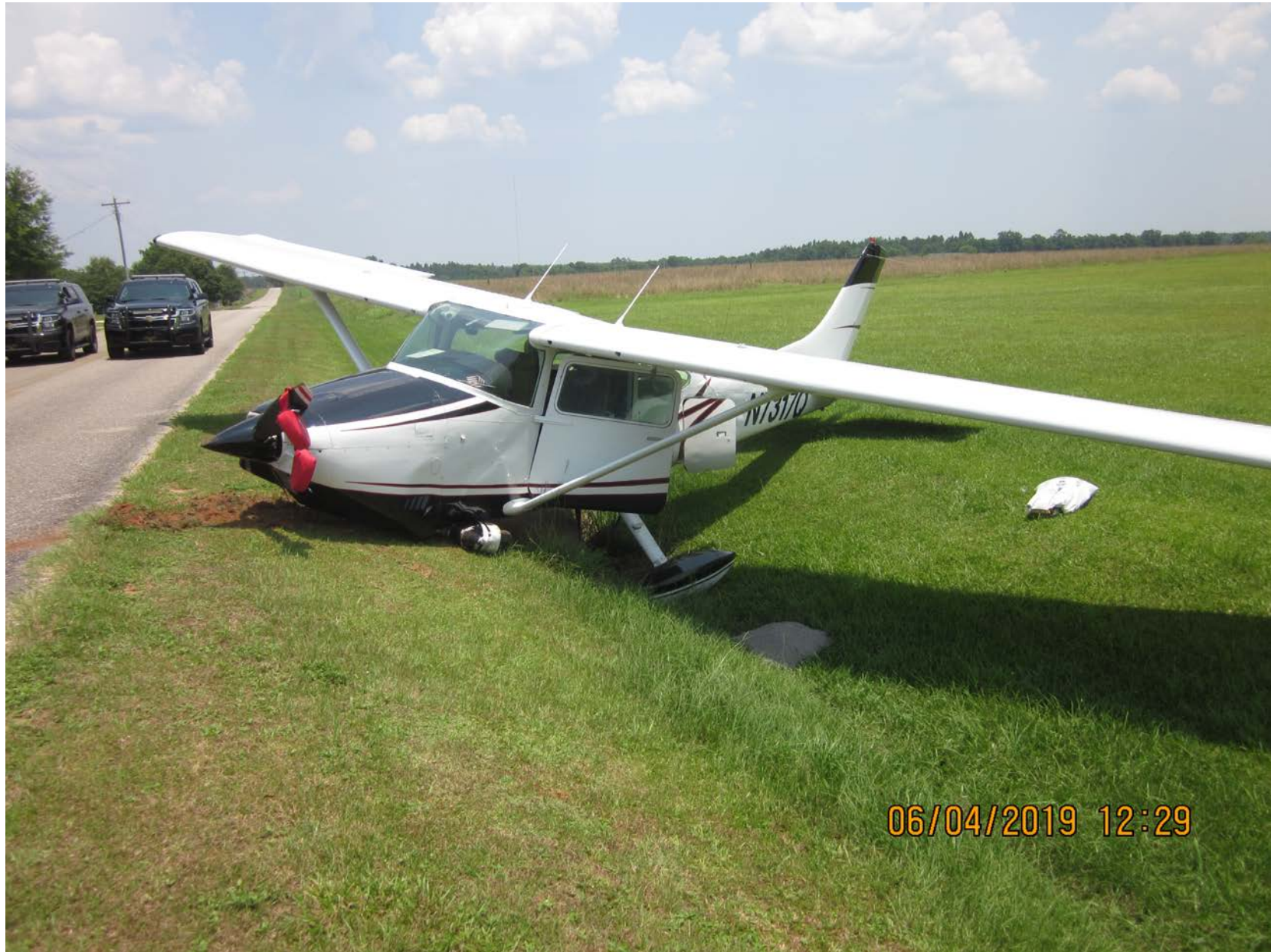
Photo 1 – View of left front quarter of airplane showing landing gear and engine cowl damage. (Courtesy of FAA)
