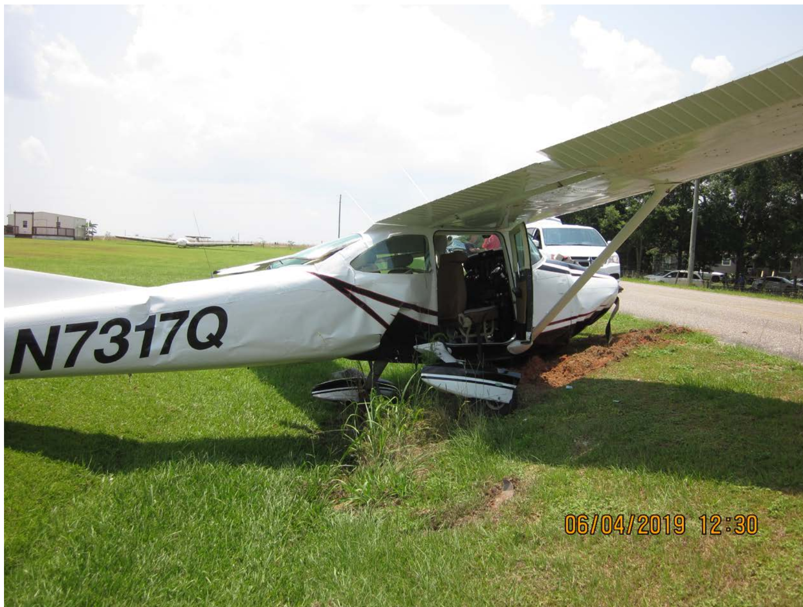
Photo 2 – View of right side of plane showing fuselage buckling and landing gear damage. (Courtesy of FAA)
