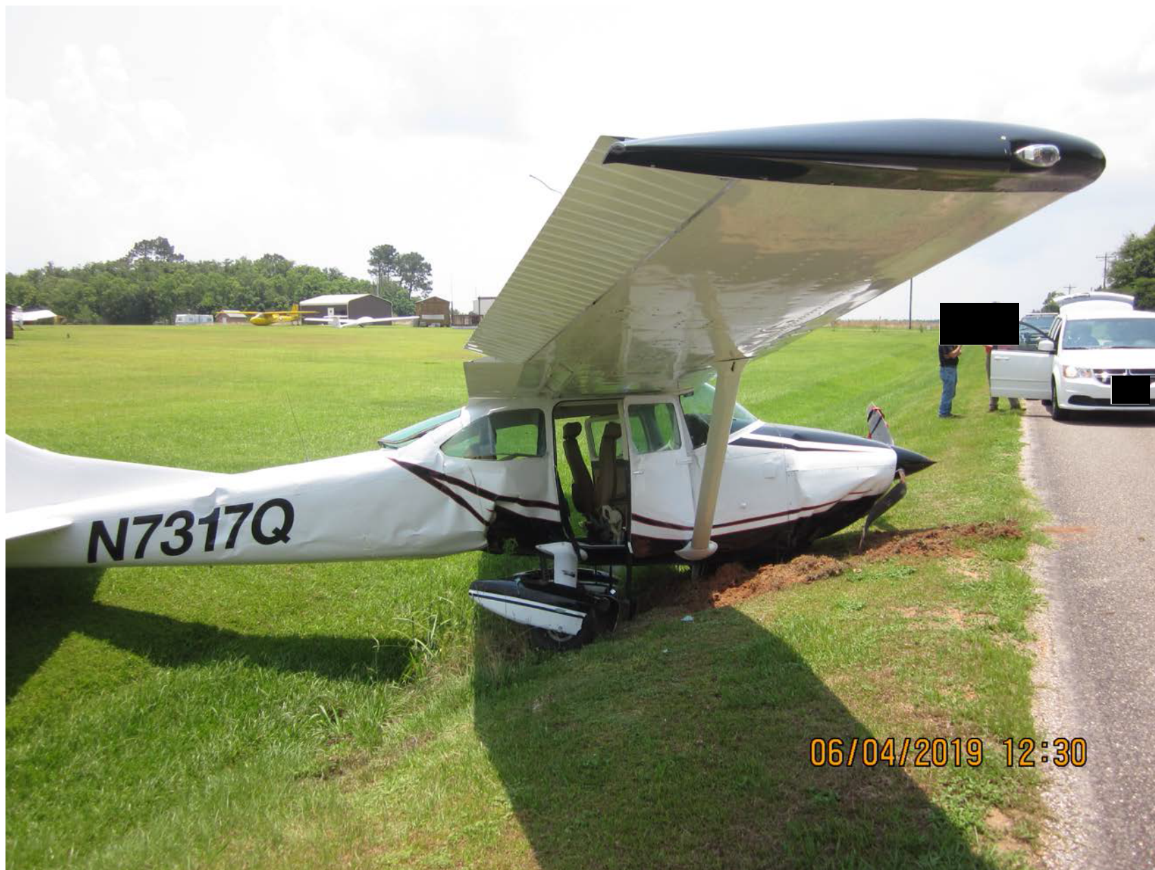
Photo 3 – Right profile view of airplane showing overall damage to fuselage and engine compartment. (Courtesy of FAA)
