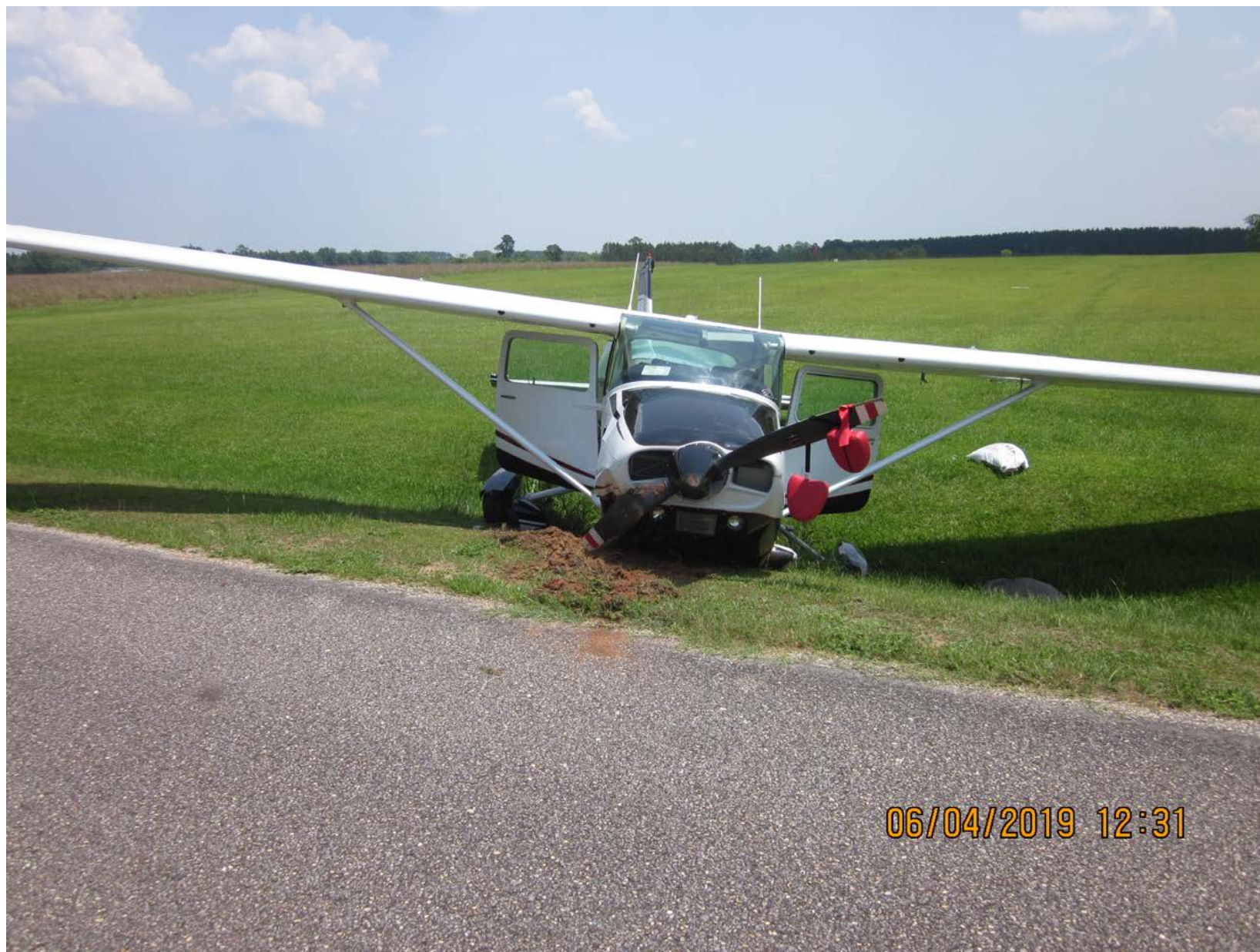
Photo 4 – View of nose of airplane showing damage to propeller and ground scars. (Courtesy of FAA)
