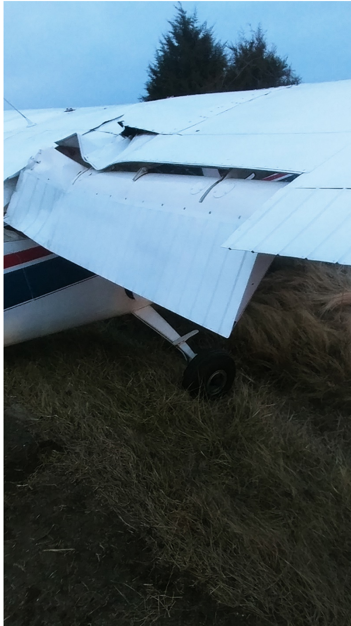
Airplane – View of Right Wing Damage (courtesy FAA)
