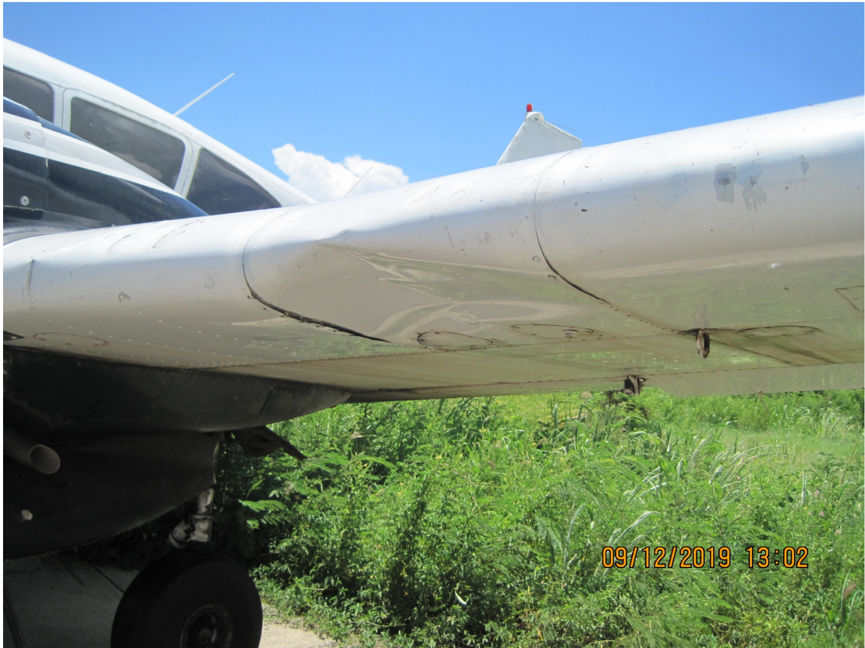
Photo 4 – Left Wing Damage (Photo Courtesy of FAA)
