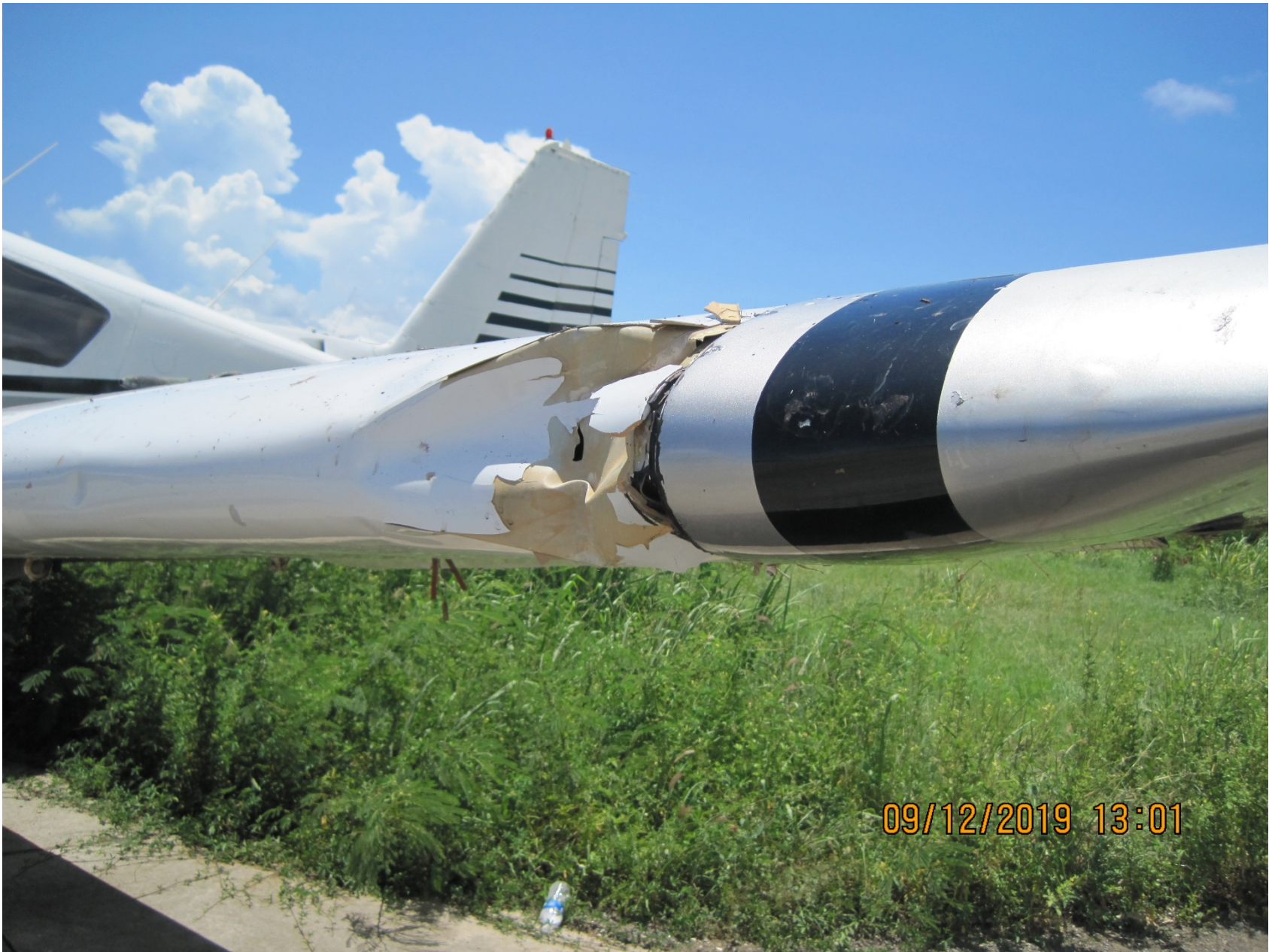
Photo 3 – View of Left Wing Fracture (Photo Courtesy of FAA)
