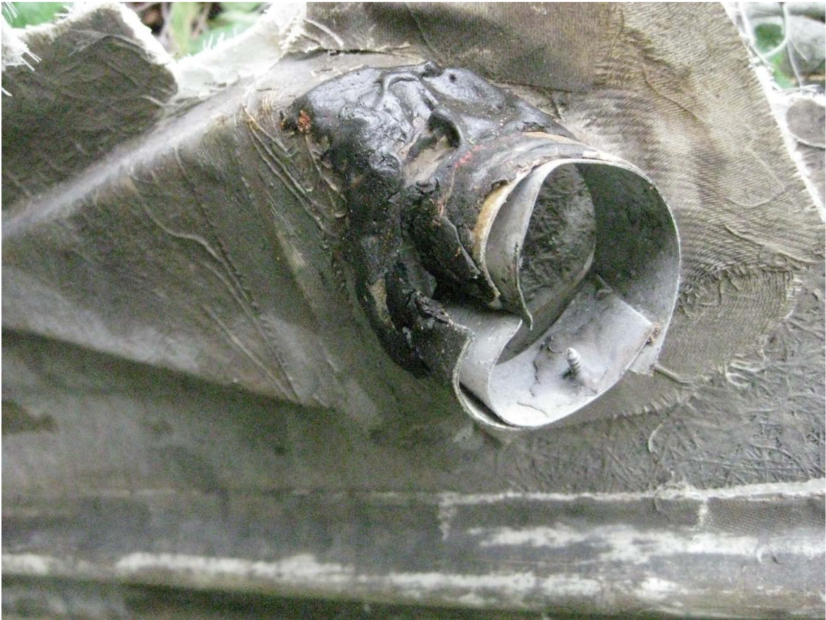
Photo 3 – View of scat tube connector on airframe intake showing crushed fitting
