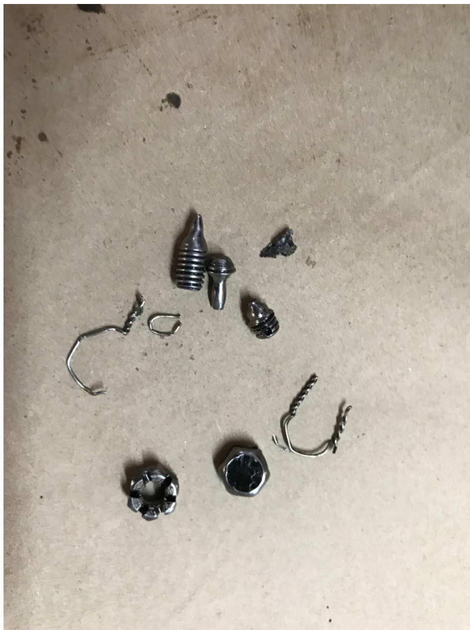
Photo 4 – Nuts, Bolts, And Safety Wire From Engine Crankshaft Idler Gear Flange (Photo Courtesy of Lycoming)
