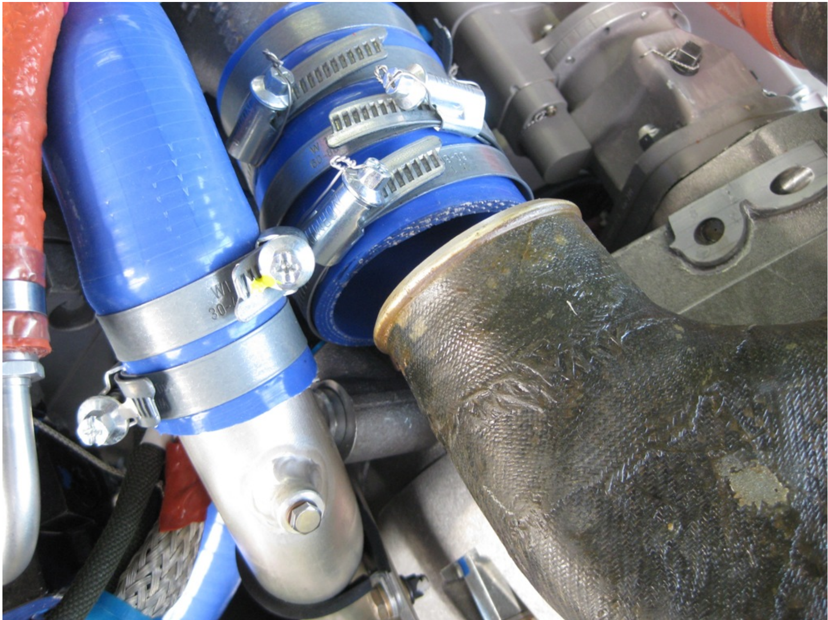
Photo 5 - Flexible induction coupling from the intercooler to the engine induction inlet. (Photo Courtesy of FAA)
